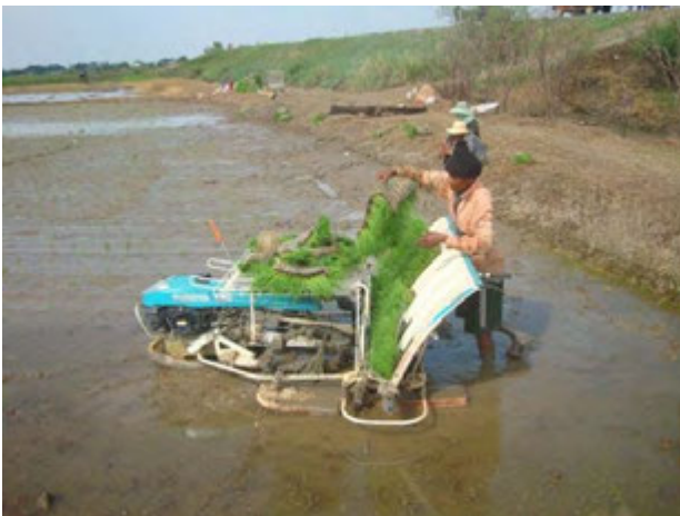
Transplanting facilitated by 6-row type machine. (Nov. 26, 2012)
