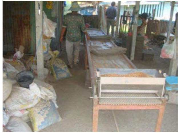
Seeding machine for nursery tray, which helps equally distribute the paddy seeds on the tray. (Nov. 10, 2012)
