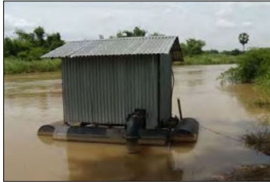
Water distribution by EPDS at Moo 1 Baan Bang Bah which is the floating canal (Bang Bah-Nong Payom)
