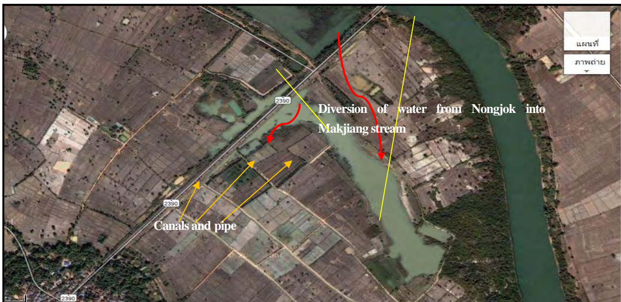
Fig 6: Water management model in Ban Yang Ngoi, Si Songkhram Sub- district, Si Songkhram district
