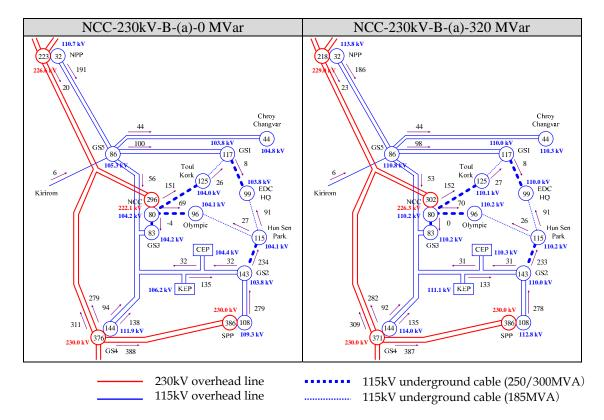
Figure 3. 26 Voltages of Phnom Penh in 2020 (SC: 0MVar / 320MVar)
