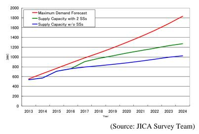
Figure 9.1 The project's Benefit: capacity increase of the Phnom Penh power grid
