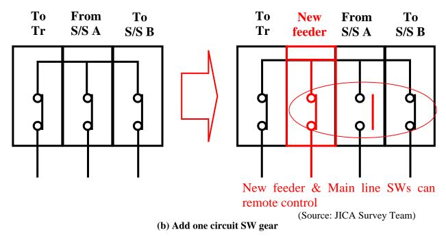
Figure 6. 22 Load Divides Method of Distribution Substation.
