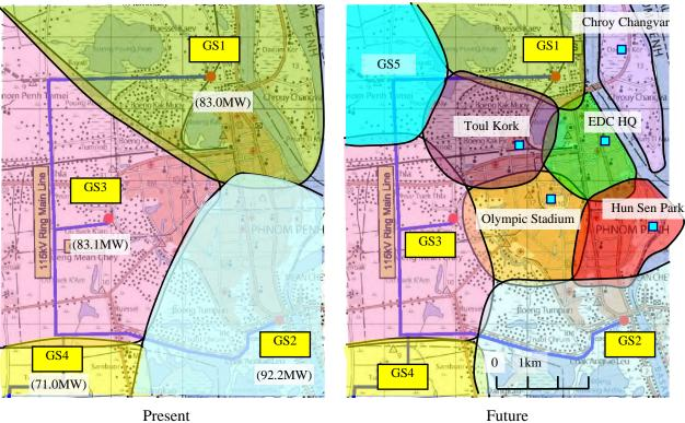
with the SPP substation, and the western and southern parts of the GS3 substation is supplied with the GS4 substation.
