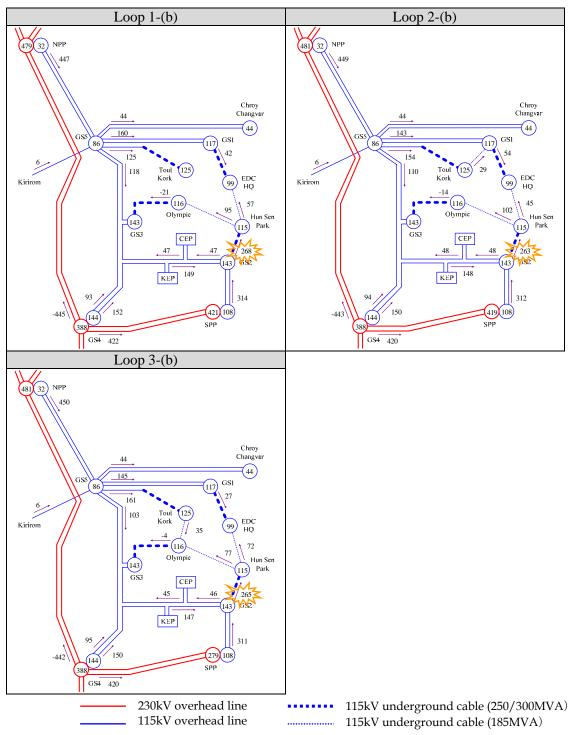
Figure 3. 22 Active Power Flow Diagram in 2020(b) (Hydro Power in Cambodia)
