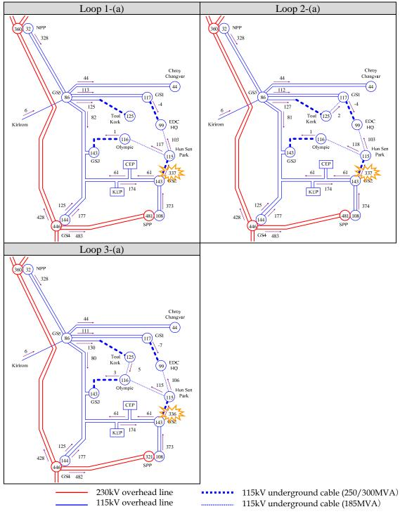
Figure 3. 21 Active Power Flow Diagram in 2020(a) (Power Import from Vietnam)
