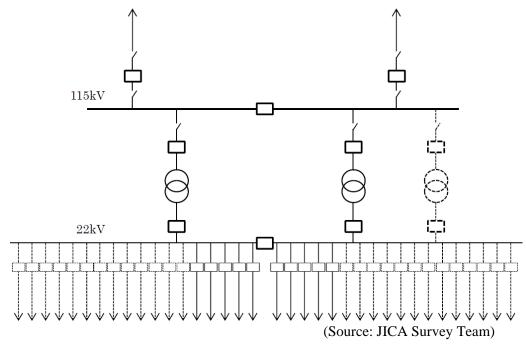
In addition, Figure 6. 18 shows a single line diagram of the substation.
