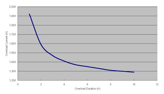
Figure 3. 19 Short Term Capacity of Triplex-type 115kV Underground Cable
