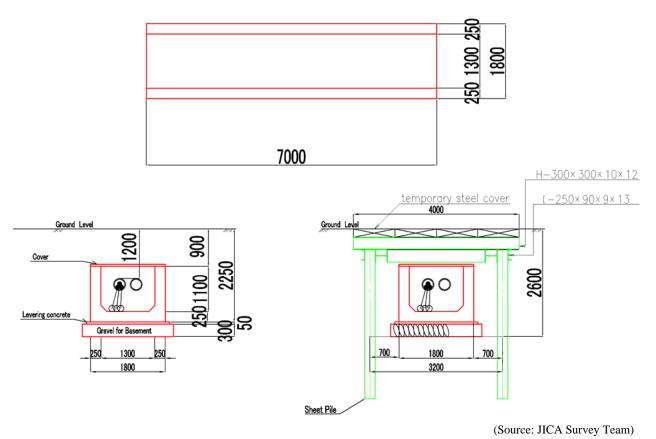
Figure 6. 12 Structure Figure and Temporary Figure of Joint Bay
