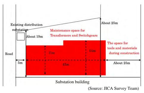
Figure 6. 16 Allocation Image of Substation Building at EDC HQ Site
