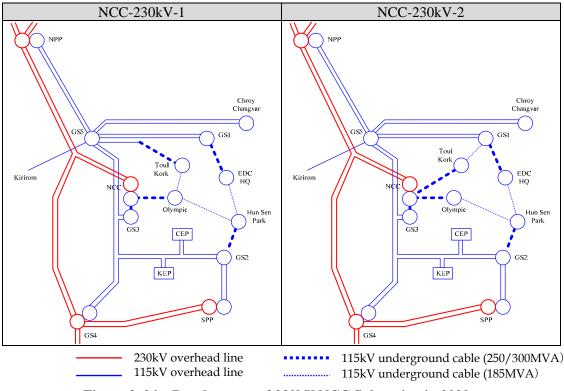
Figure 3. 24 Development of 230kV NCC Substation in 2020
