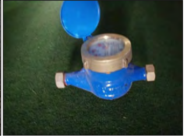
Photo-4 Water meter
