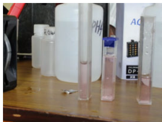
(4) Checking reliability of chlorine test kits and reagents (Right: JICA test kit (new), Middle: WHO test kit, Left: JICA Test kit (Old), Right and middle showed almost same color:
