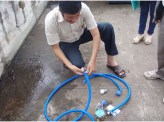
Examination of instrumental error with reference (standard) water meter
