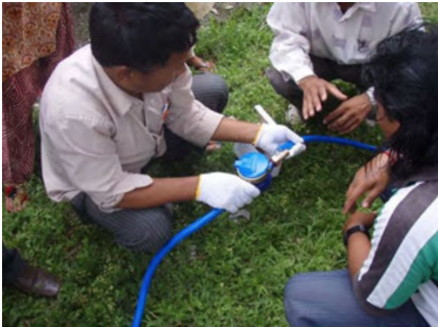
Examination of instrumental error with reference (standard) water meter for Dhulabari WUSC's water meter
