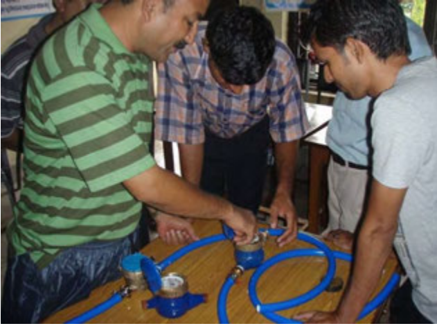
Examination of instrumental error with reference (standard) water meter for Mangadh WUSC's water meter
