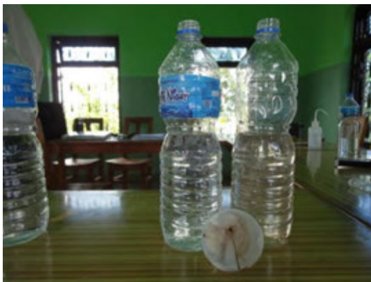
(9) Right bottle: Filtrate just after backwash (pink), Left bottle: Filtrate after 10 minutes from backwashing, Front: Residue by filtration (Gauradaha WUSC)
