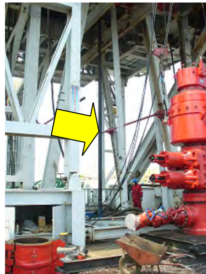
Drilling (kelly in the middle)
