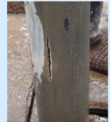
Crack on Drilling Pipe
