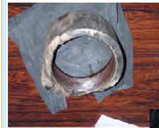
Broken Sub – upper part
