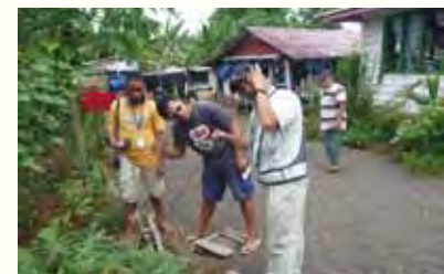
Detecting the sounds of leakage with a meter
