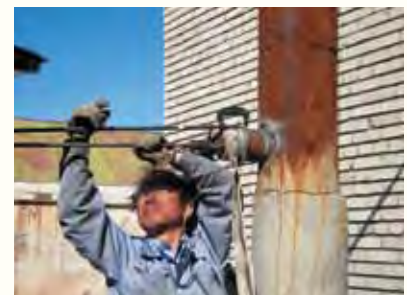
Measuring emission gas density in smoke stack
