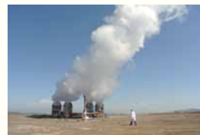
Geothermal steam production testing in Menengai, Kenya
