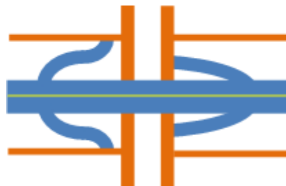
C4: Half Interchange Type (half diamond)
