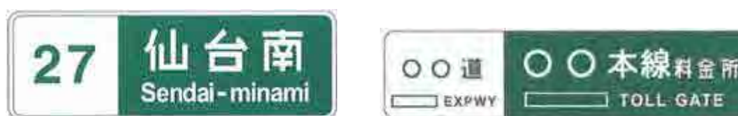
Figure 11.44 Signs of interchange and toll plazas on toll booth roof
