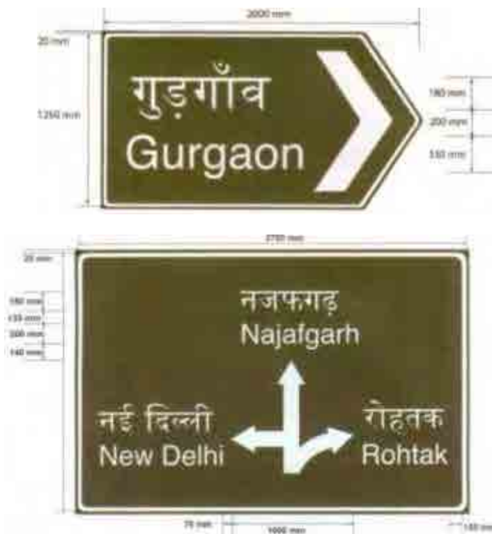
Figure 11.2 Standardized size of Direction Sign (Indian standards)
