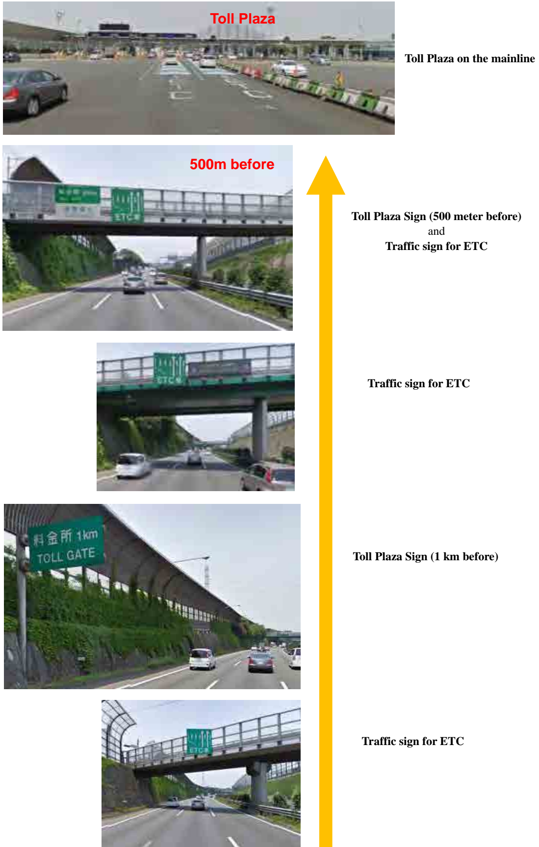
Figure 11.30 Exit to Toll Plaza (Example of Diamond interchange in Japan)
