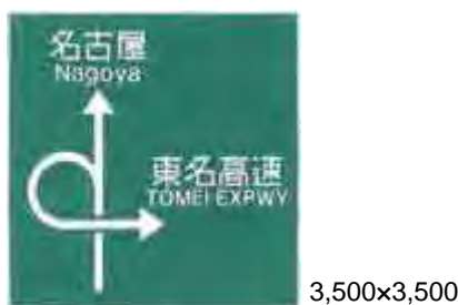
Figure 11.5: Map-type Guide sign for IC Entrance (Japanese Expressway Standard)
