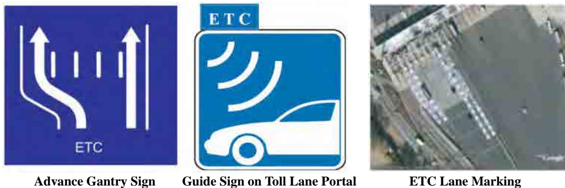
Figure 11.45: Signage and Marking for ETC (Indian Standards)
