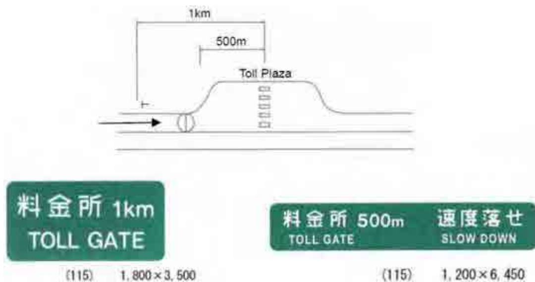
Figure 11.29: Guide Traffic Signs for Toll Plaza in Japan
