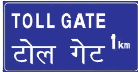
Figure 11.27: Toll Plaza Sign
