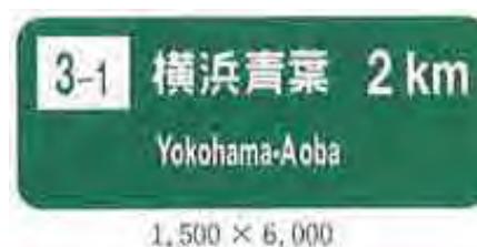
Figure 11.18: Exit Guide Sign, 109 sign
