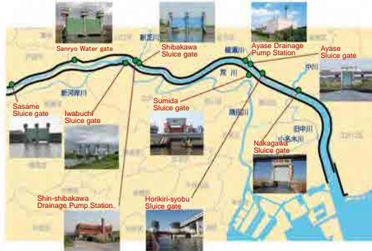
River structures requiring seismic strengthening (sluiceways)
