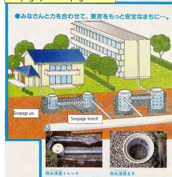
Seepage pits • Seepage trench
