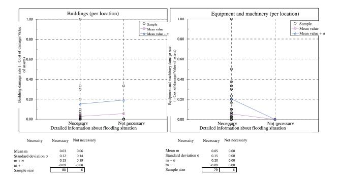
Diagram 1-4: Correlation between Need for Flood Alerts and Damage Rates (Detailed Information about Flooding Situation 2)
