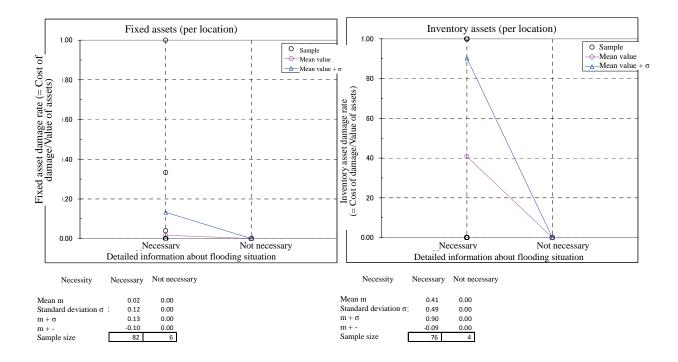
Diagram 1-3: Correlation between Need for Flood Alerts and Damage Rates (Detailed Information about Flooding Situation 1)
