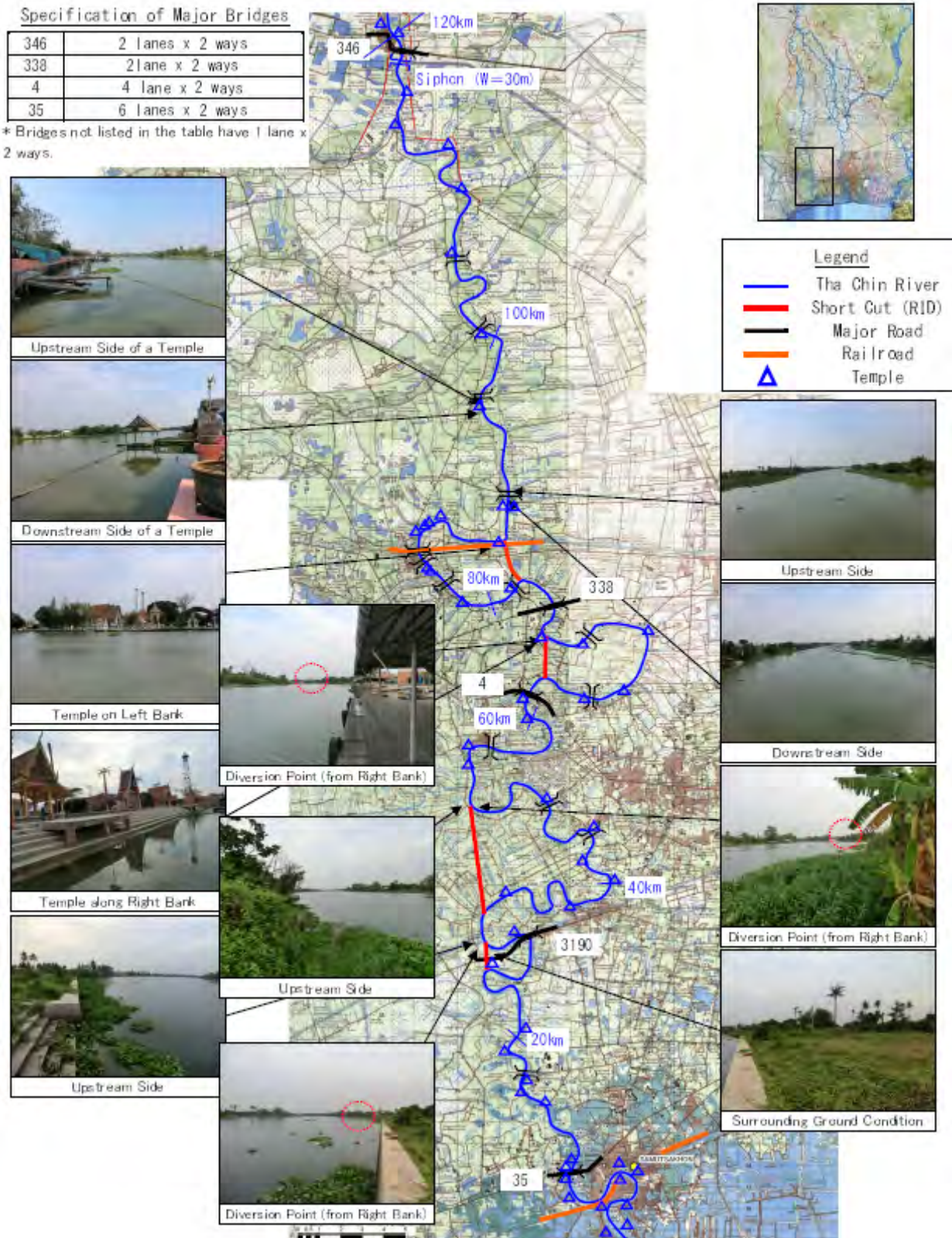
Figure Q2.5.6 Planning Area (Gulf of Thailand to Route 346, Approx. 119km long) -Dike Improvement and Short Cut Channels in the Tha Chin River Basin-
