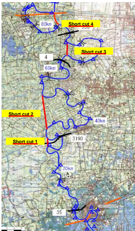
Figure 11.3.6 Planning Area (Short Cut Channels) - Dike Improvement and Short Cut Channels in the Tha Chin River Basin -
