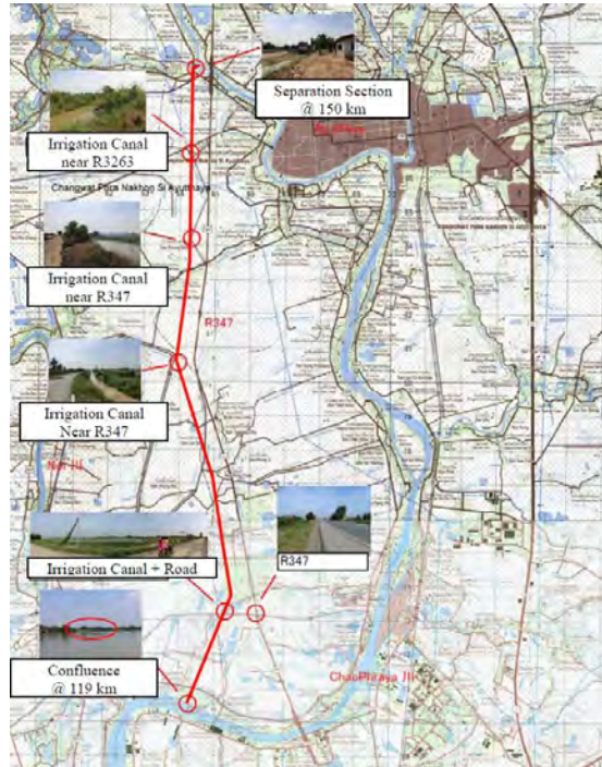
Figure 10.2.48 Bypass Channel Planned along Route 347
