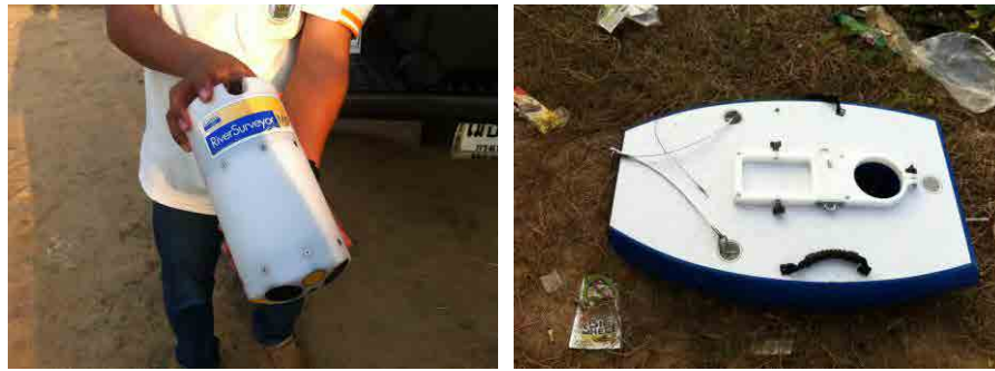
Figure 7.2.1 River Surveyor M9 (V-ADCP) prepared by RID
