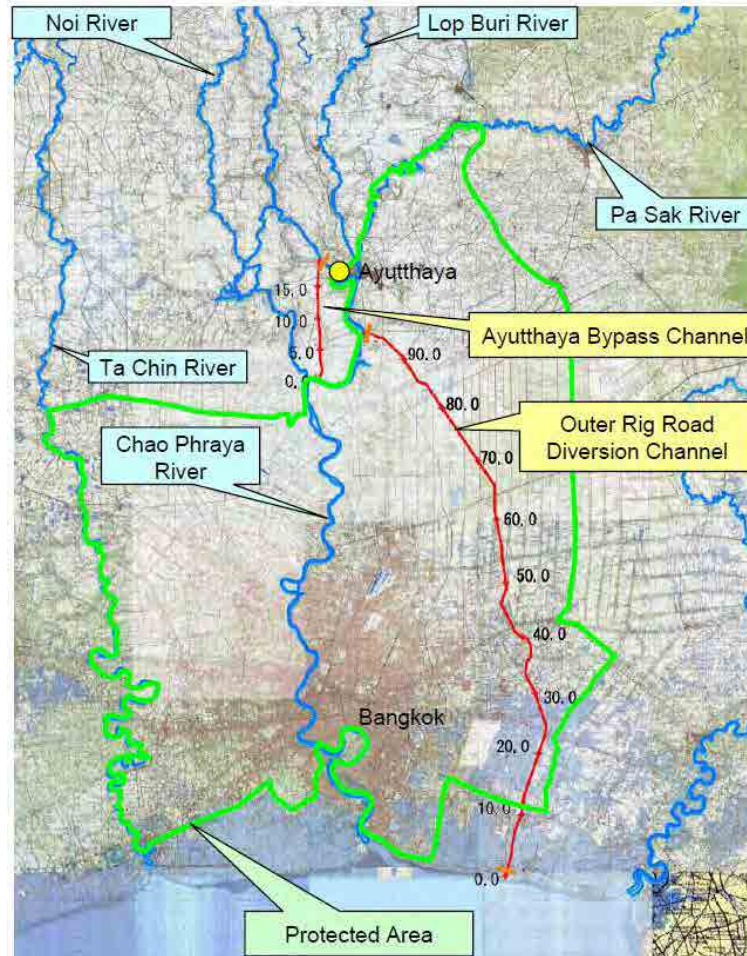
Figure 5.3.1 Proposed Outer Ring Road Diversion Channel
