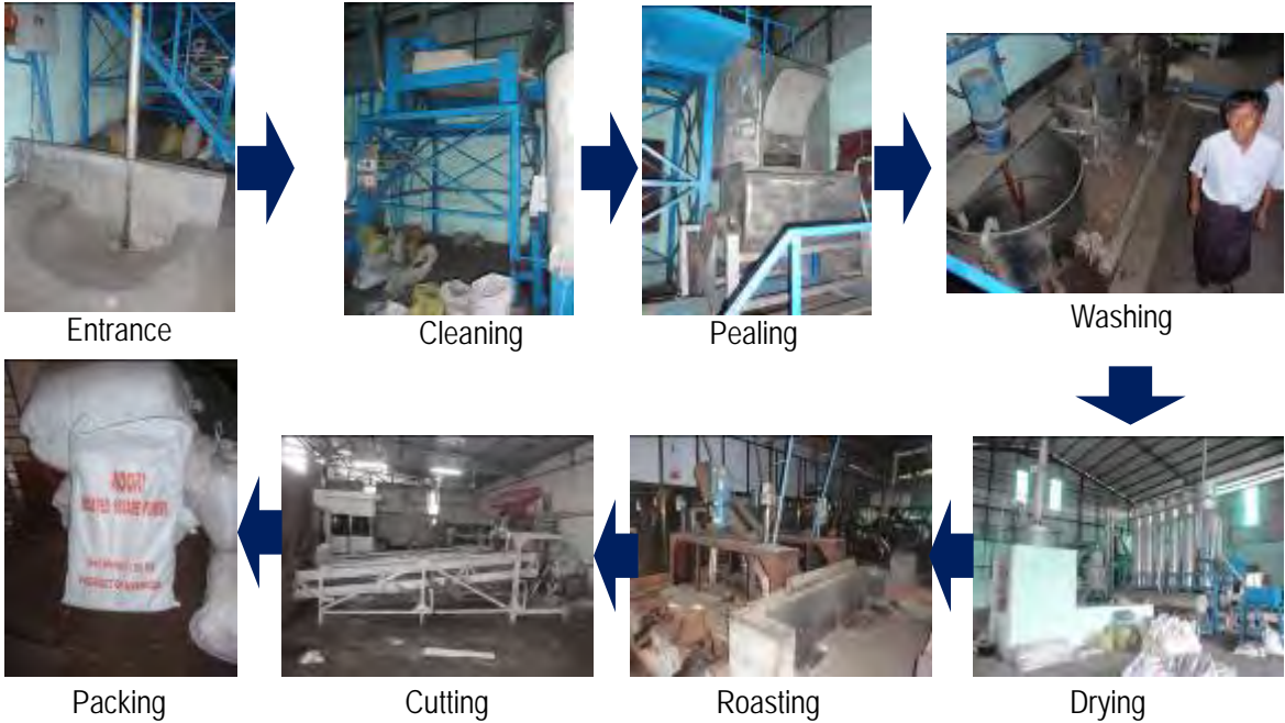
Production Process of Roasted Sesame Powder (Magway)
