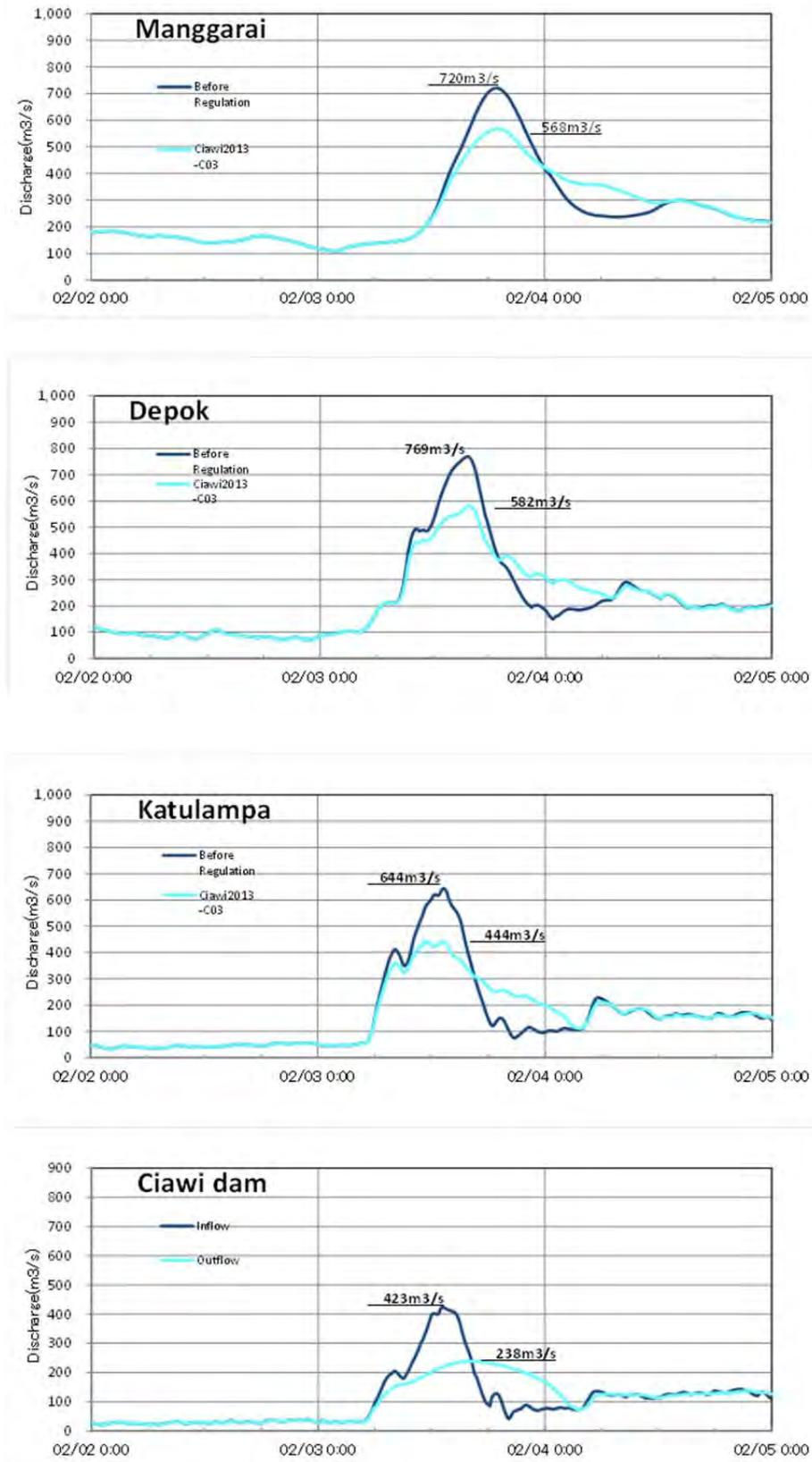
Figure 6.3-38 Ciawi Dam-1: Hydrographs of Flood Control Points in Case 3 Flood
