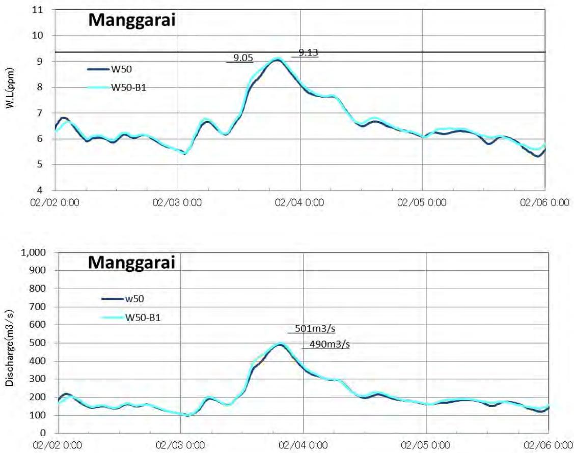
**Figure 7.3-6 Water Level and Discharge Hydrograph (B1 Scenario)**
