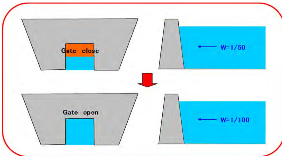
Figure 6.3-20 Image of Service Outlet Design
