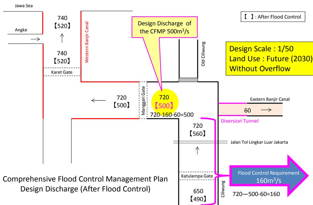
Figure 6.1-1 Design Flood Discharge Allocation
