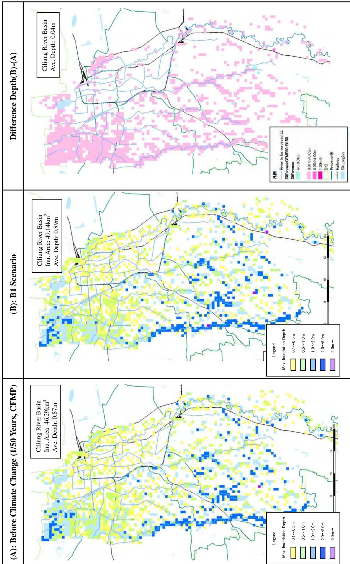
Figure 7.3-8 Comparison of Inundation Conditions before Climate Change and B1 Scenario
