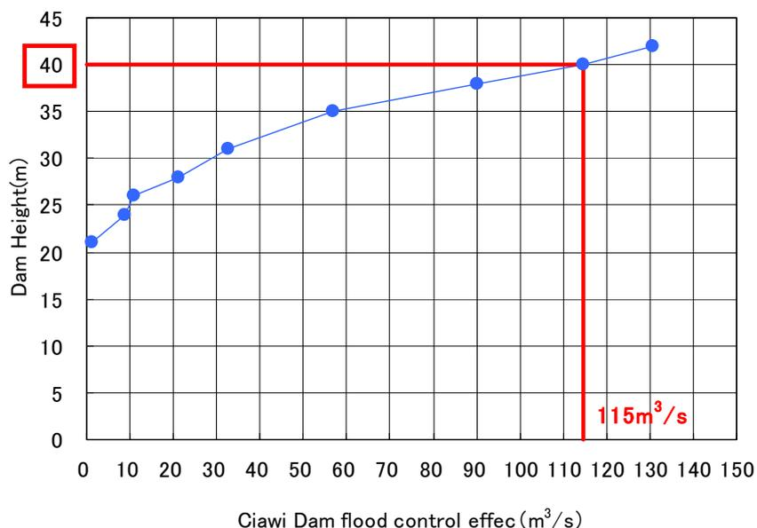
Figure 6.3-30 Dam Height and Flood Control Effect of Ciawi Dam-1 at Dam Site
