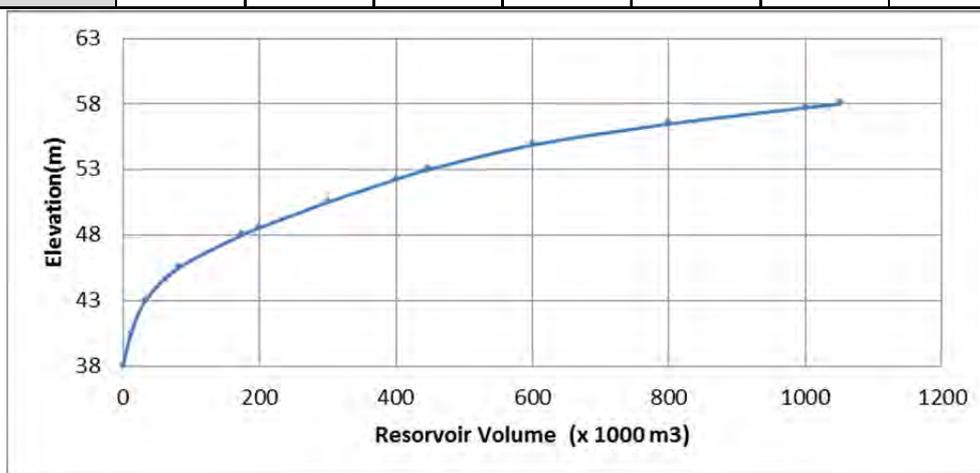
**Figure 6.5-1 H-V Curve of Pesona Kayangn Gate Dam**
