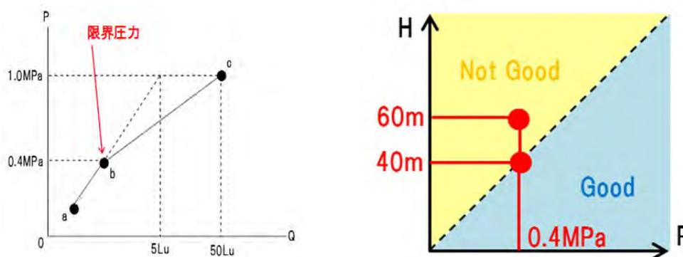
Figure 6.3-12 Limit Pressure by P-Q Curve
