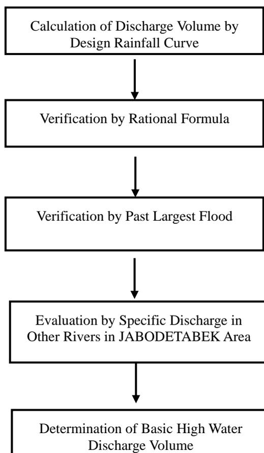
**Figure 5.3-10 Determination Flow of Basin Design Discharge Volume**
