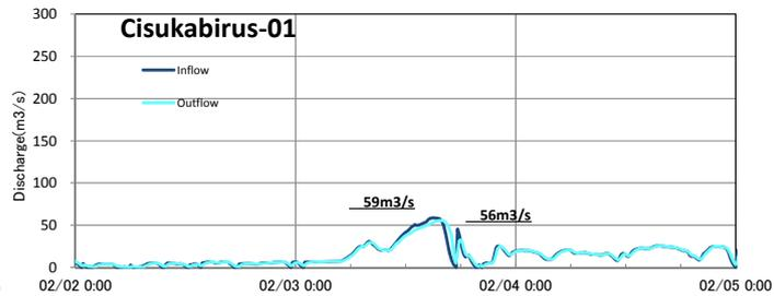
Figure 6.3-39 Ciawi Dam 2 + Cisukabirus Dam: Hydrographs of Flood Control Points in Case 1 Flood
