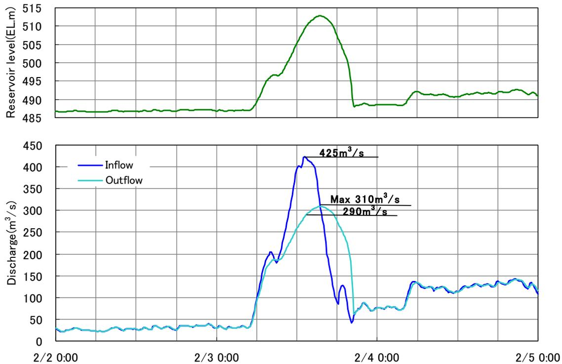
Figure 6.3-25 Hydrograph of Ciawi Dam-1
