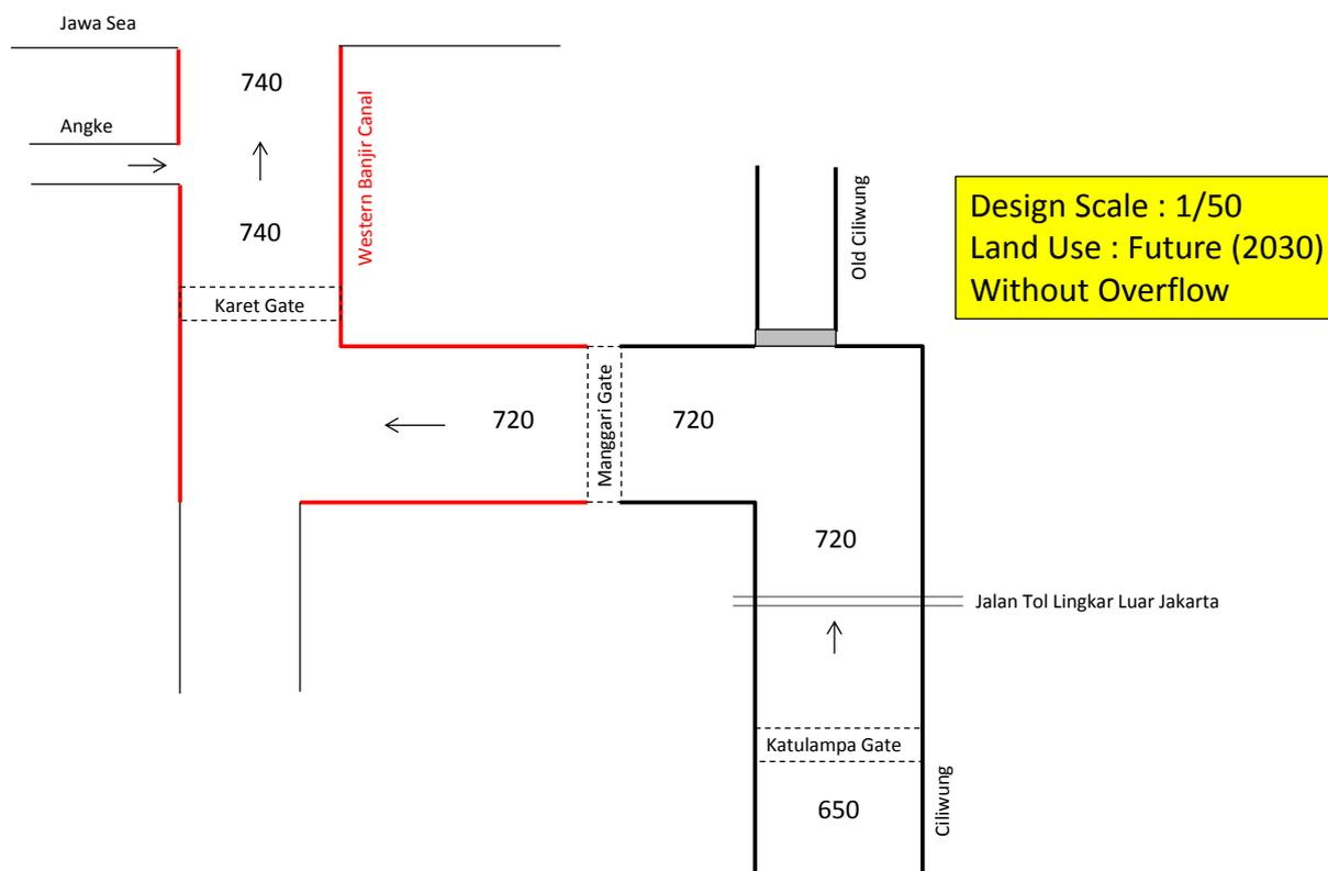
**Figure 5.3-15 Allocation of Basin Design Discharge Volume**
