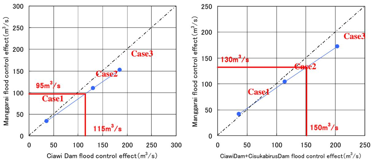
Figure 6.3-35 Relation of Flood Control Effects between Dam Sites and Flood Control Points
