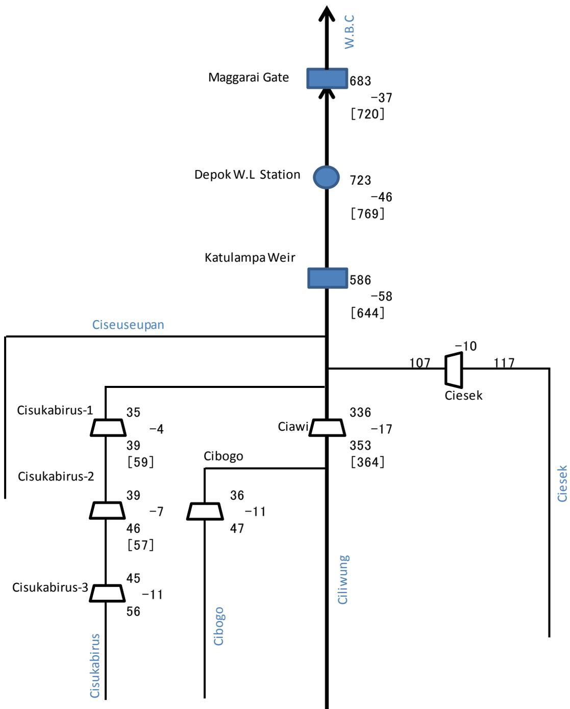
Figure 6.4-4 Flood Discharge Allocation
