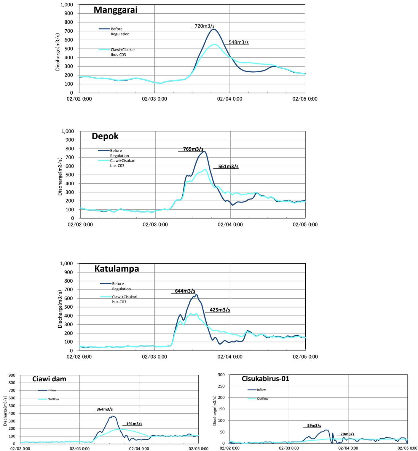
Figure 6.3-41 Ciawi Dam 2 + Cisukabirus Dam: Hydrographs of Flood Control Points in Case 3 Flood
