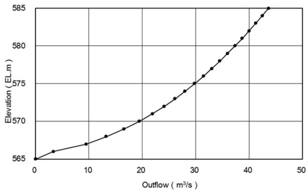
Figure 6.3-21 Outflow Characteristics of Proposed Dams
