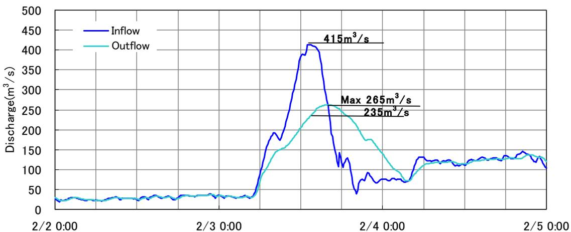
Figure 6.3-28 Hydrograph of Ciawi Dam-2 + Cisukabirus Dam
