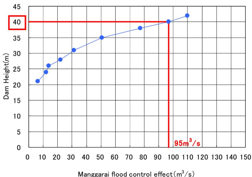
Figure 6.3-31 Dam Height and Flood Control Effect of Ciawi Dam-1 at Manggarai
