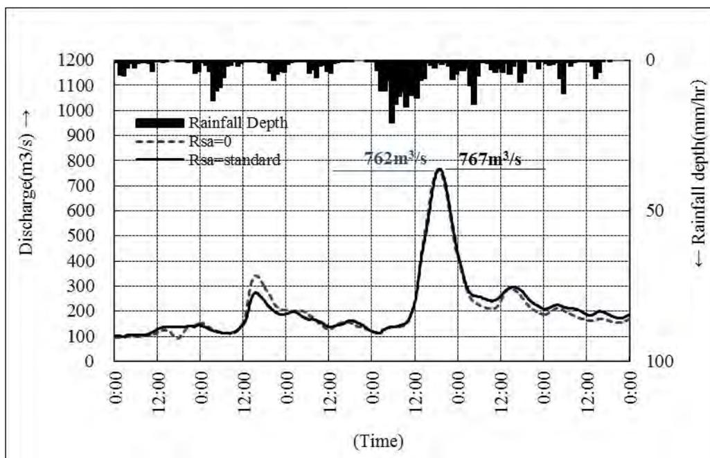
**Figure 5.3-12 Hydrograph at Manggarai Point (Largest Recorded Flood: February 2007, Loss of Rainfall: Design Value, Saturation Value)**
