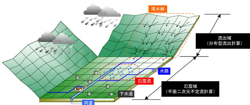
**Figure 8.2-1 Image of Flood Analysis Model using Distributed Type**
