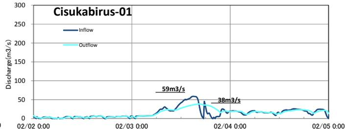
**Figure 6.3-40** Ciawi Dam 2 + Cisukabirus Dam: Hydrographs of Flood Control Points in Case 2 Flood
