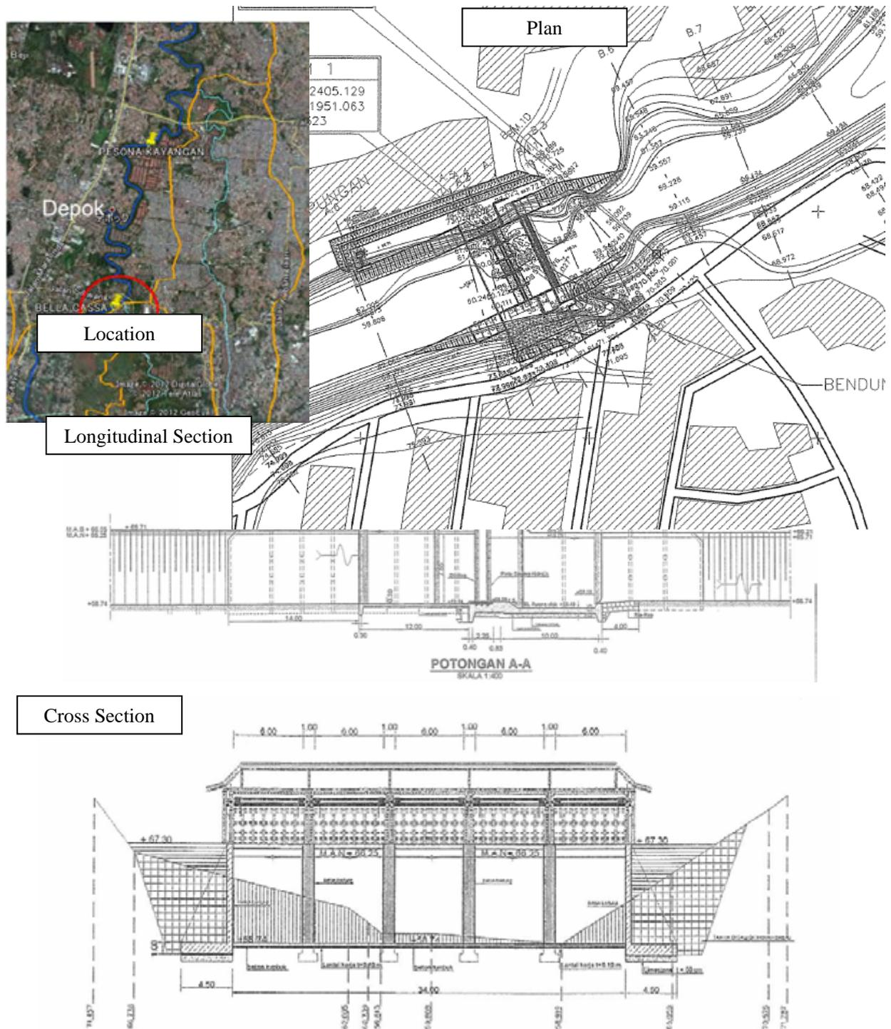
Figure 6.5-4 Design of Bella Cassa Gate Dam
