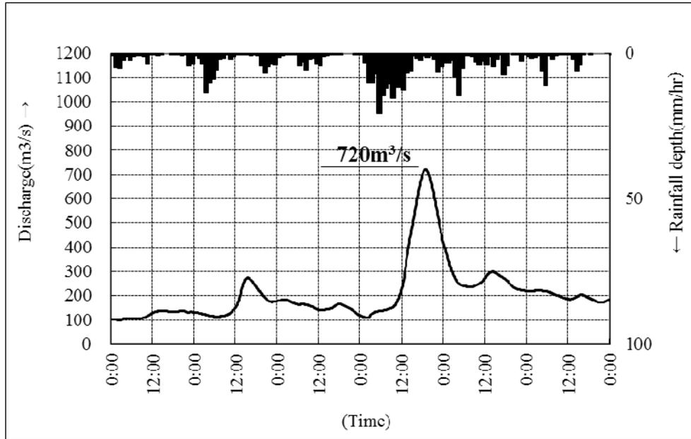
**Figure 5.3-11 Hydrograph at Manggarai Point (Design Discharge: Flood Type on 30 January 2007)**
