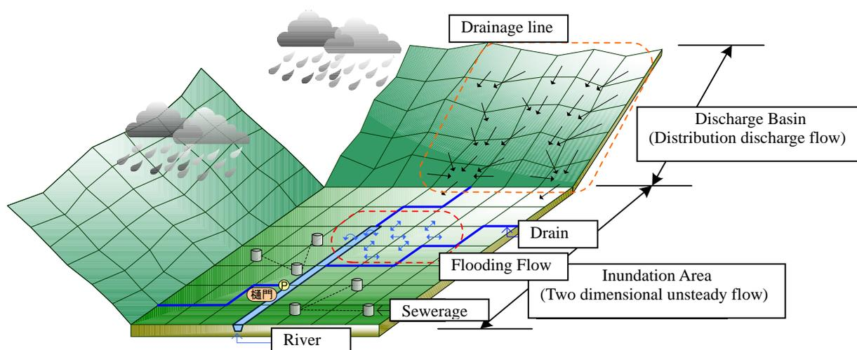
Figure 5.3-5 Image of Flood Inundation Analysis Model
