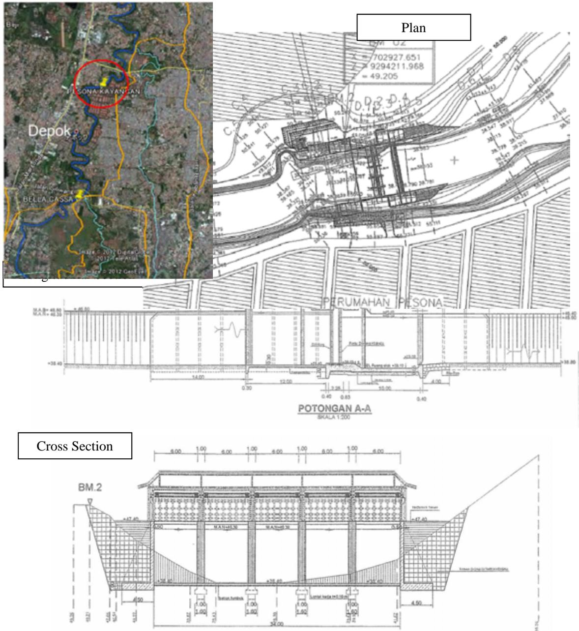
Figure 6.5-3 Design of Pesona Kayangan Gate Dam
