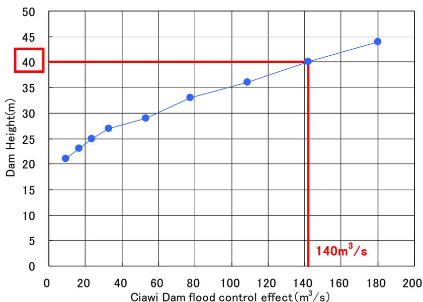
Figure 6.3-32 Dam Height and Flood Control Effect of Ciawi Dam-2 at Dam Site
