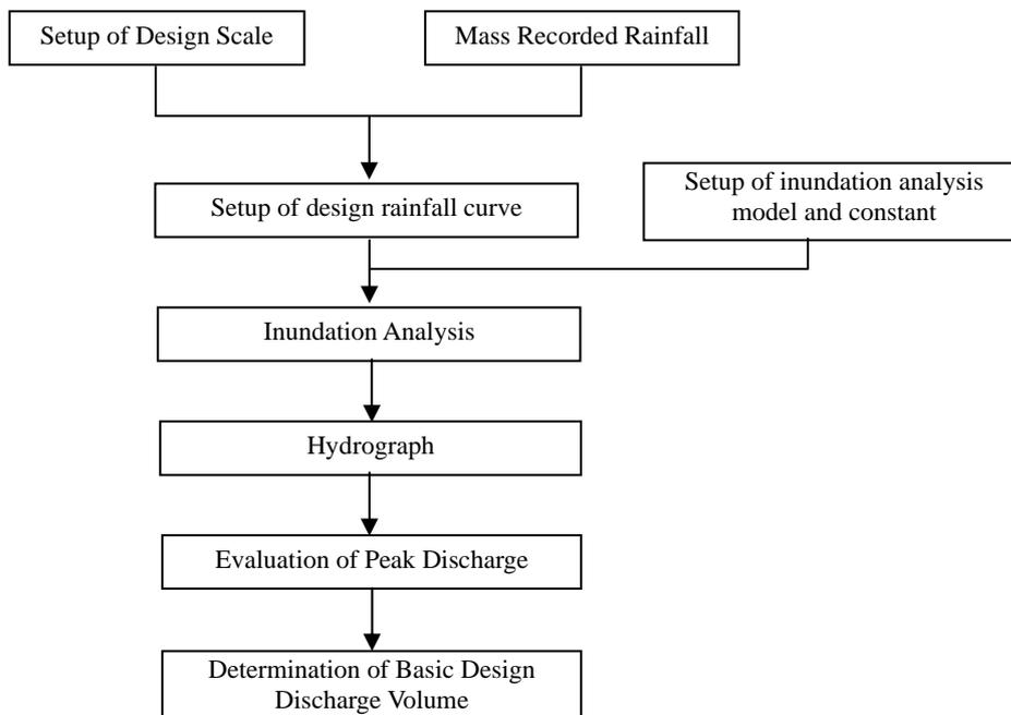
**Figure 5.3-1 Flow Chart of Basin Design Discharge Volume Examination**
