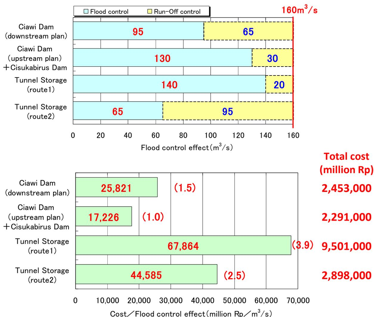
Figure 6.7-1 Flood Control Effects and Costs of Large Dams and Tunnel Storage
