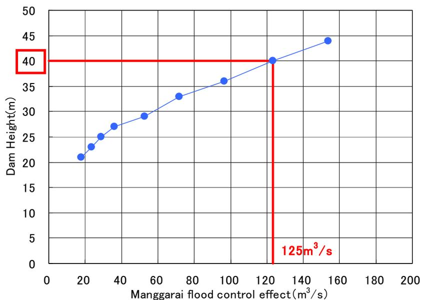
Figure 6.3-33 Dam Height and Flood Control Effect of Ciawi Dam-2 at Manggarai
