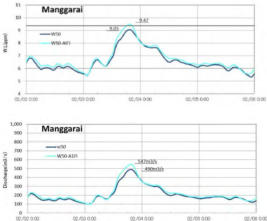
**Figure 7.3-9 Water Level and Discharge Hydrograph (A1FI Scenario)**
