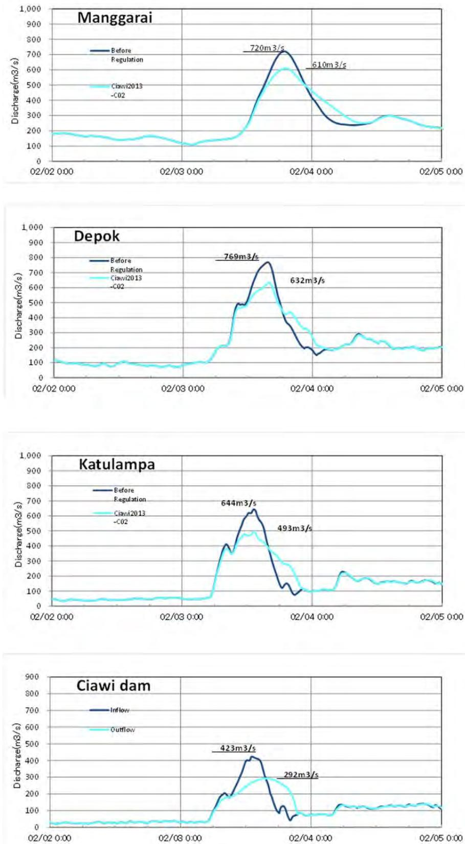
Figure 6.3-37 Ciawi Dam-1: Hydrographs of Flood Control Points in Case 2 Flood
