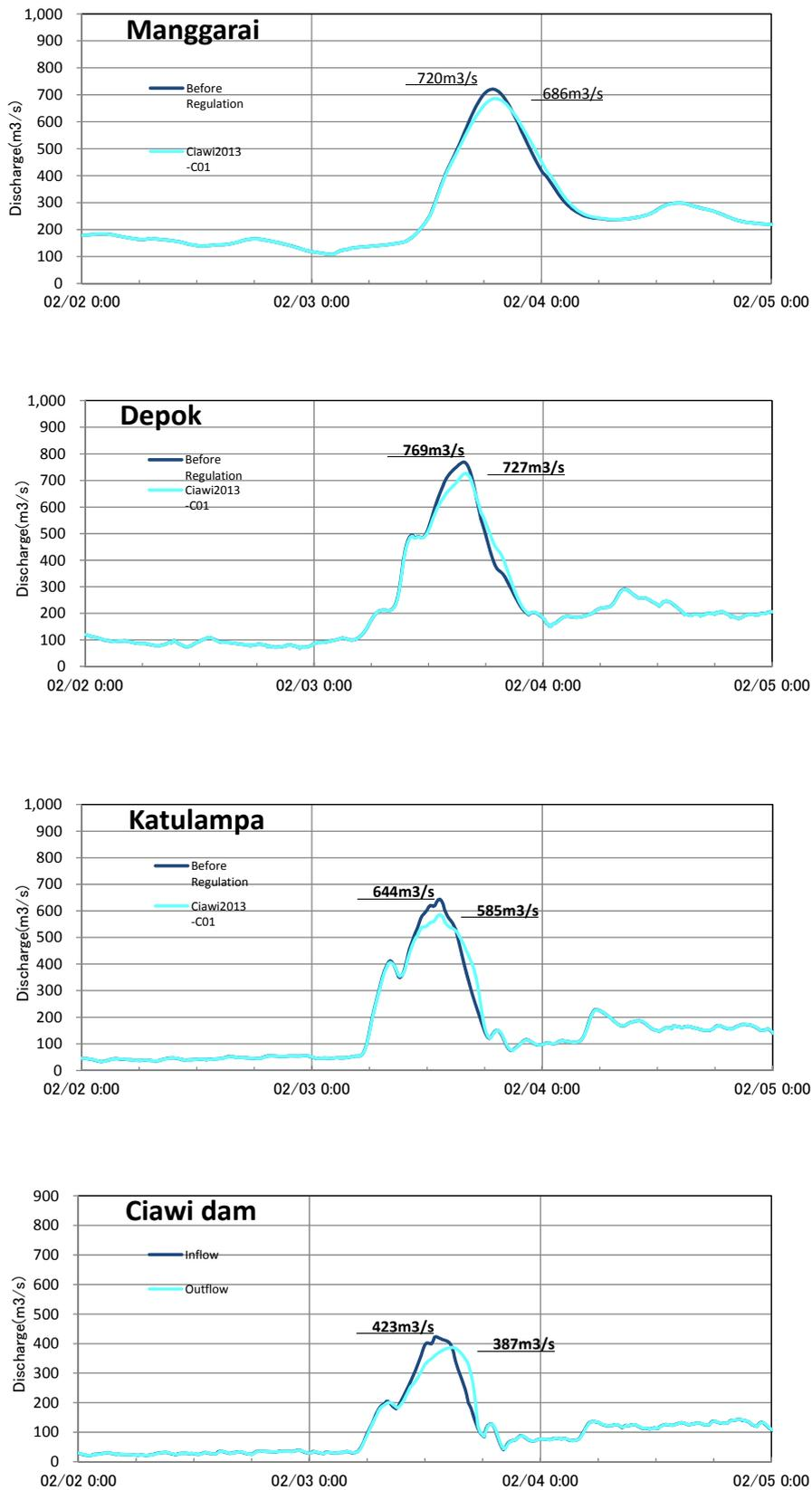
Figure 6.3-36 Ciawi Dam-1: Hydrographs of Flood Control Points in Case 1 Flood
