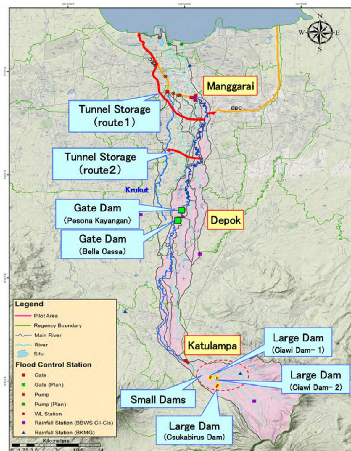
Figure 6.2-1 Locations of Candidate Flood Control Facilities in Ciliwung River
