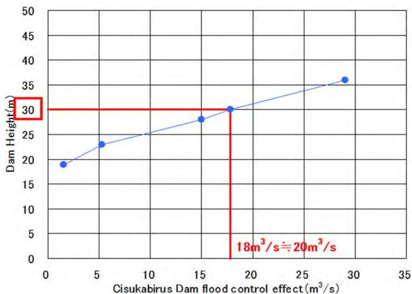
Figure 6.3-34 Dam Height and Flood Control Effect of Cisukabirus Dam at Manggarai
