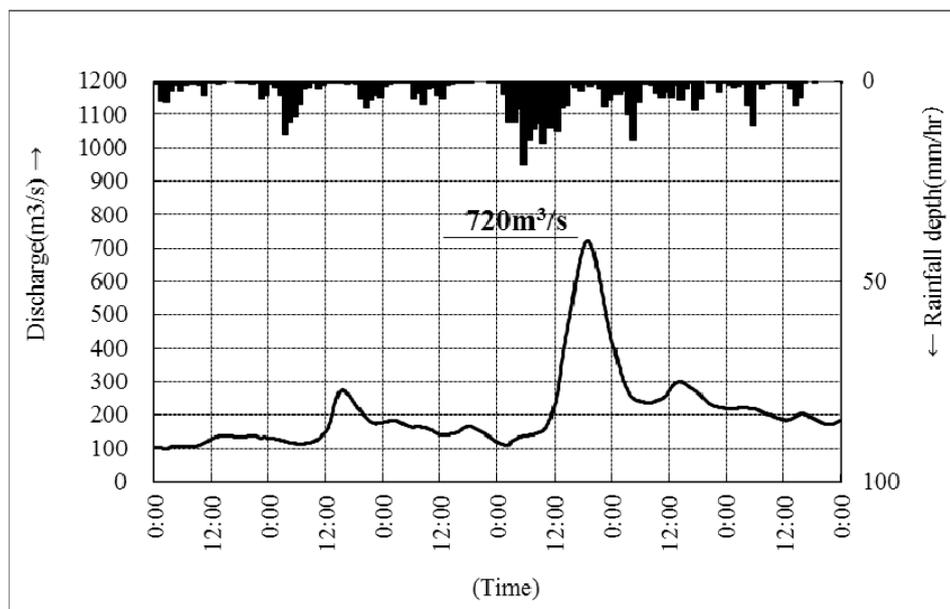
**Figure 5.3-14 Hydrograph at Manggarai Point (Design Rainfall: Flood Type on 30 January 2007)**
