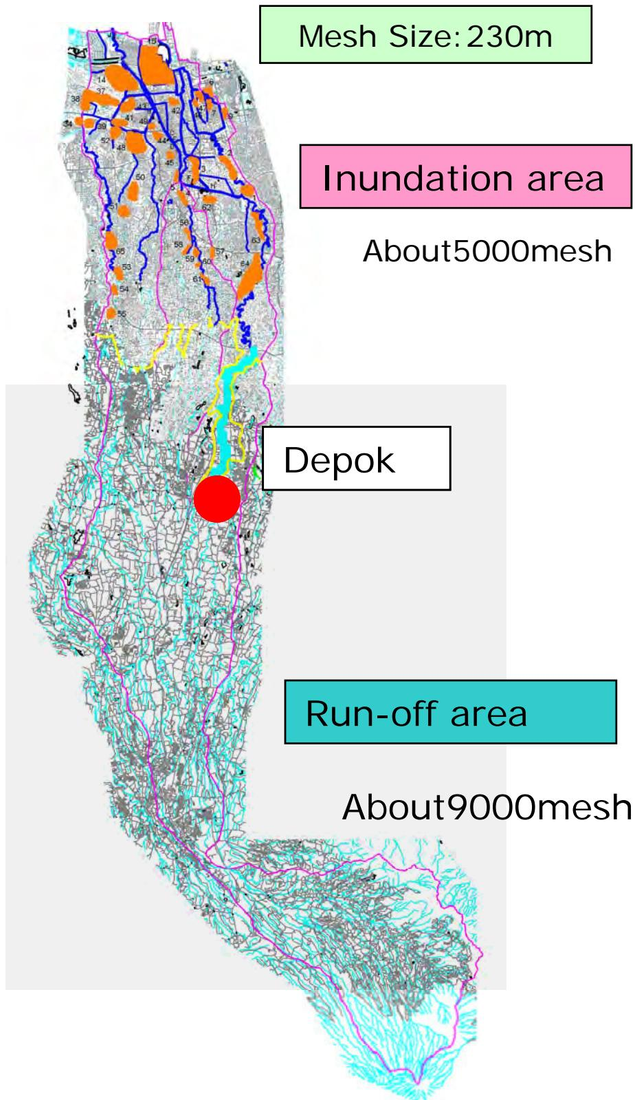
**Figure 3.2-4 Settlement of Discharge Basin and Inundation Area**
