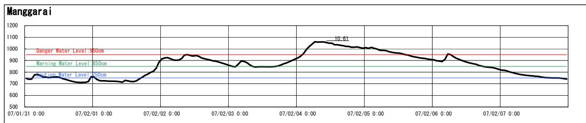
Figure 1.4-8 Hyetograph and Hydrograph (Flood in February 2007)
