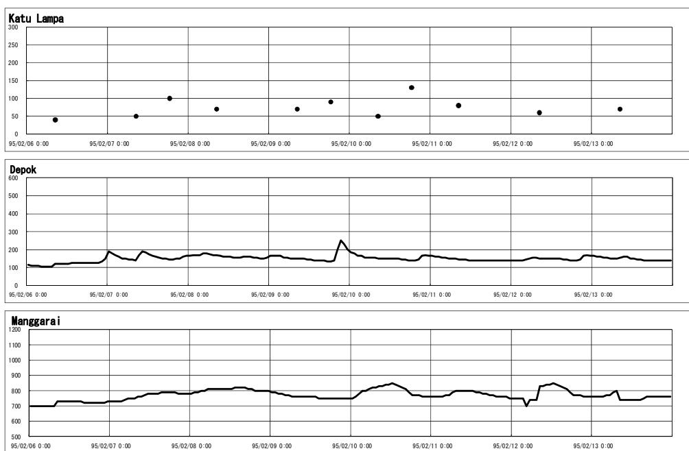
**Figure 2.4-6 Observed Water Level (Inundation in February 1995)**
