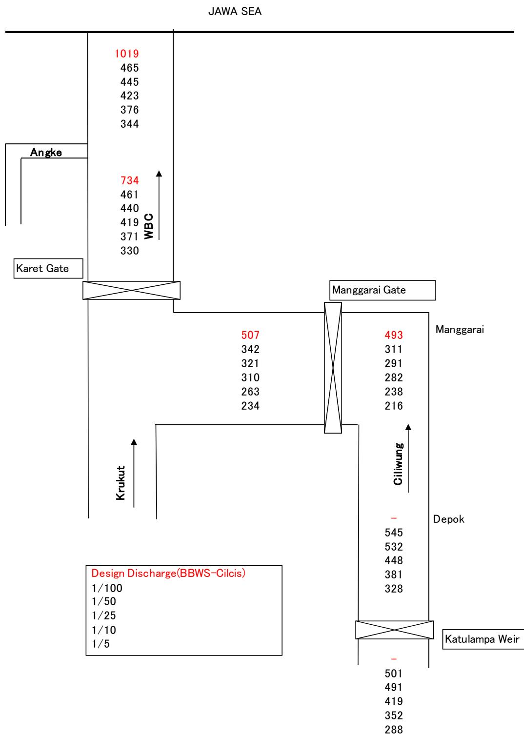
Figure 3.3-6 Discharge Distribution Map with Different Design Discharge
