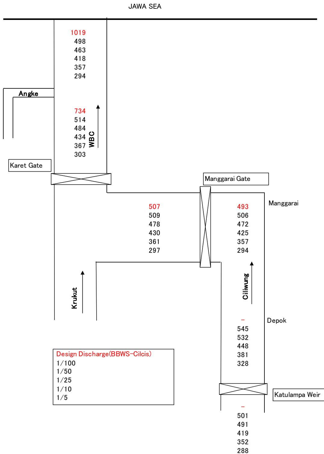
Figure 3.3-2 Discharge Distribution Map with Different Design Discharge
