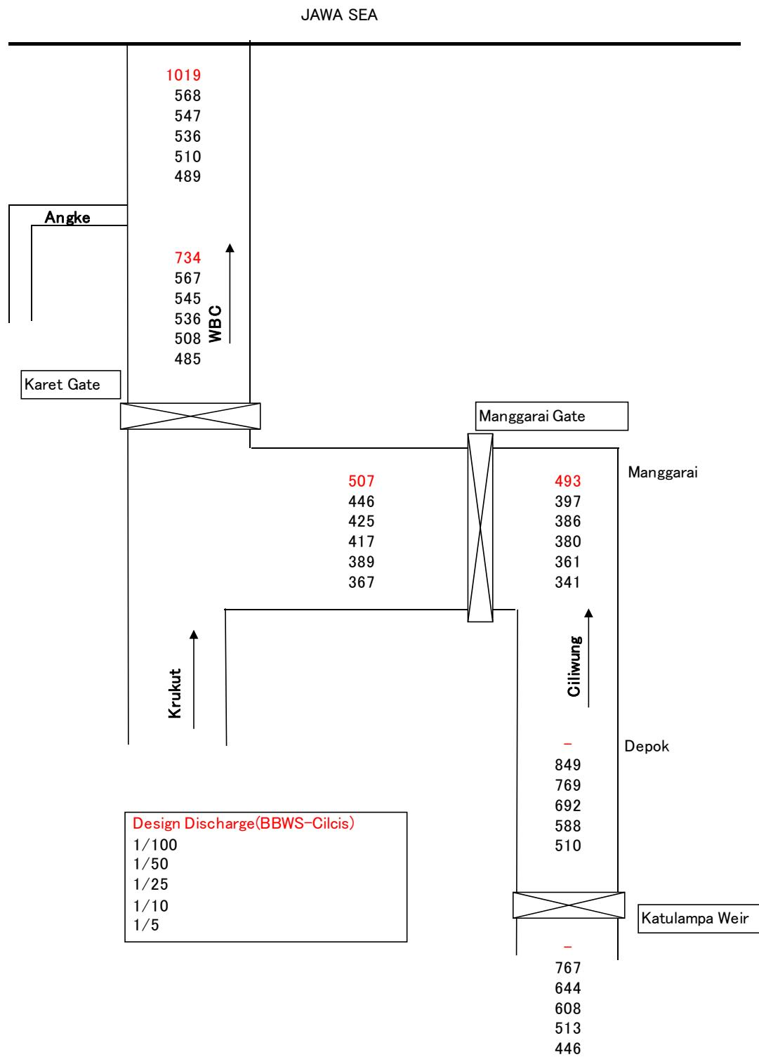
**Figure 3.3-8 Discharge Distribution Map with Different Design Discharge (Future Land Use, with Inundation, Current River Condition)**
