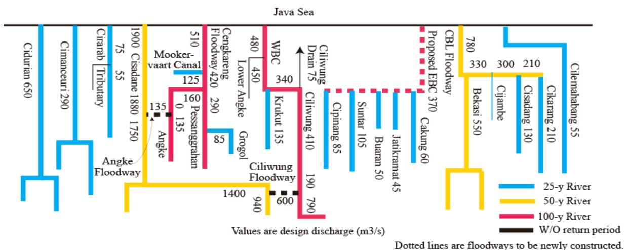
**Figure 1.5-3 Allocation Plan of Water Discharge and Safety Level of Flood Control in the Master Plan in 1997**
