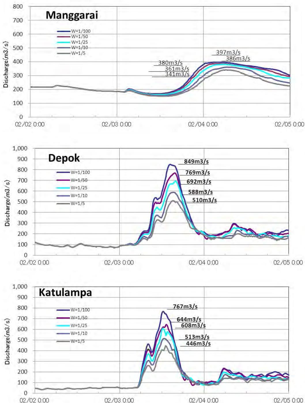
**Figure 3.3-9 Discharge Volume Hydro with Different Design Discharge (Future Land Use, with Inundation, Current River Condition)**
