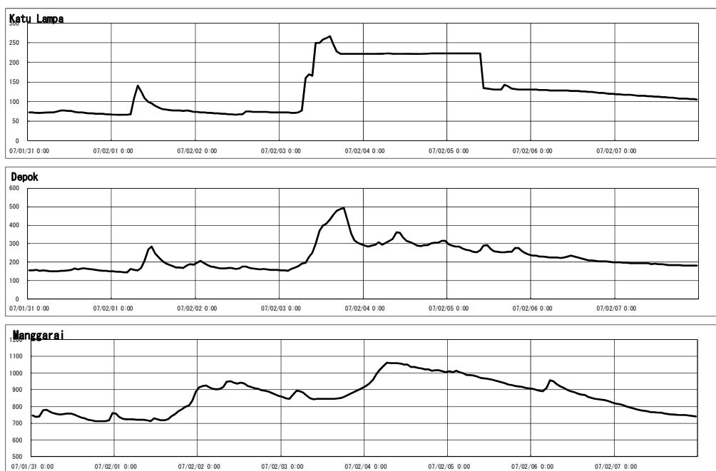
**Figure 2.4-30 Observed Water Level (Inundation in January 2007)**
