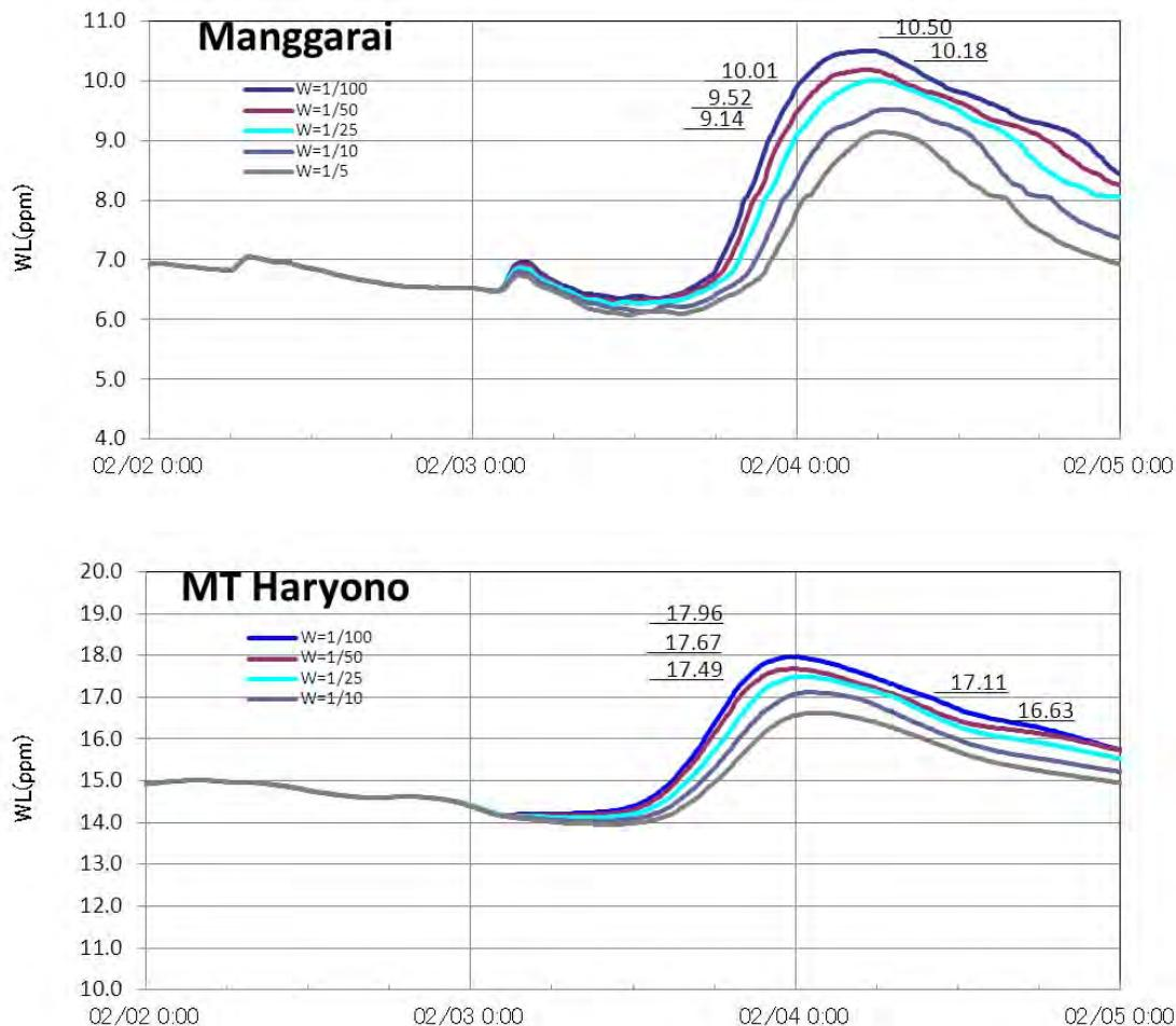
**Figure 4.3-6** River Water Level Hydro with Different Design Discharge (Current River Condition, Future Land Use)
