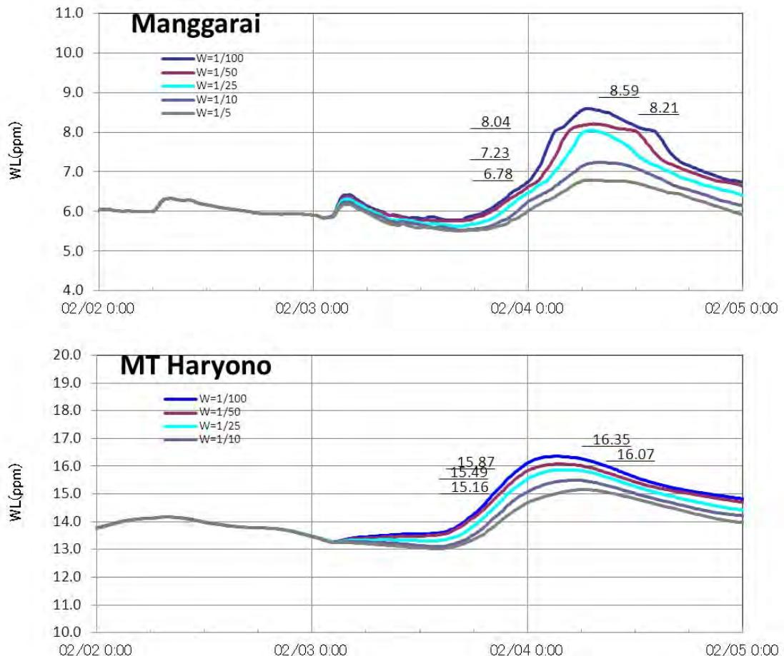
**Figure 4.3-2 River Water Level Hydro with Different Design Discharge (Current River Condition, Current Land Use)**
