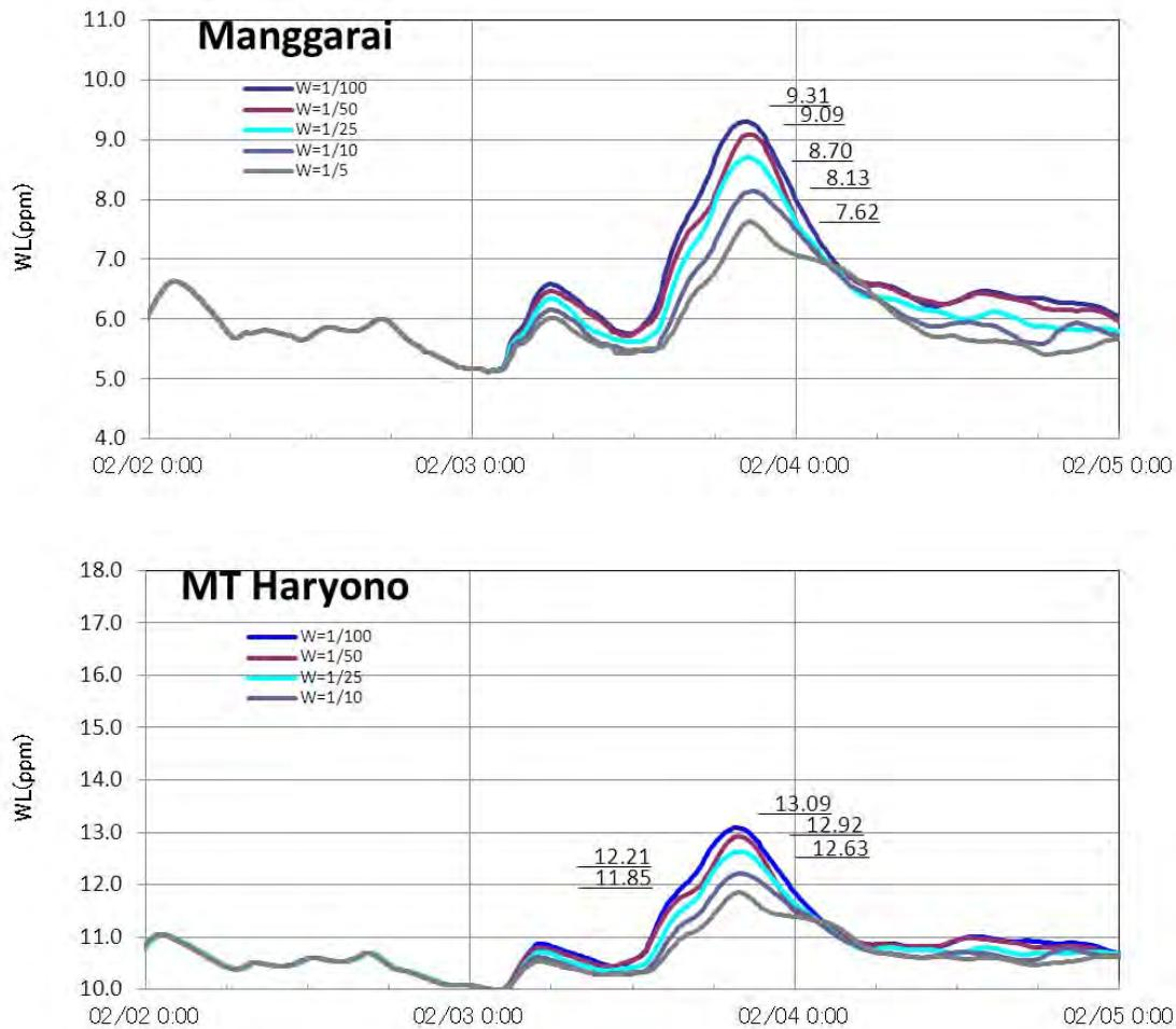
**Figure 4.3-10 River Water Level Hydro with Different Design Discharge (After River Improvement, Current Land Use)**
