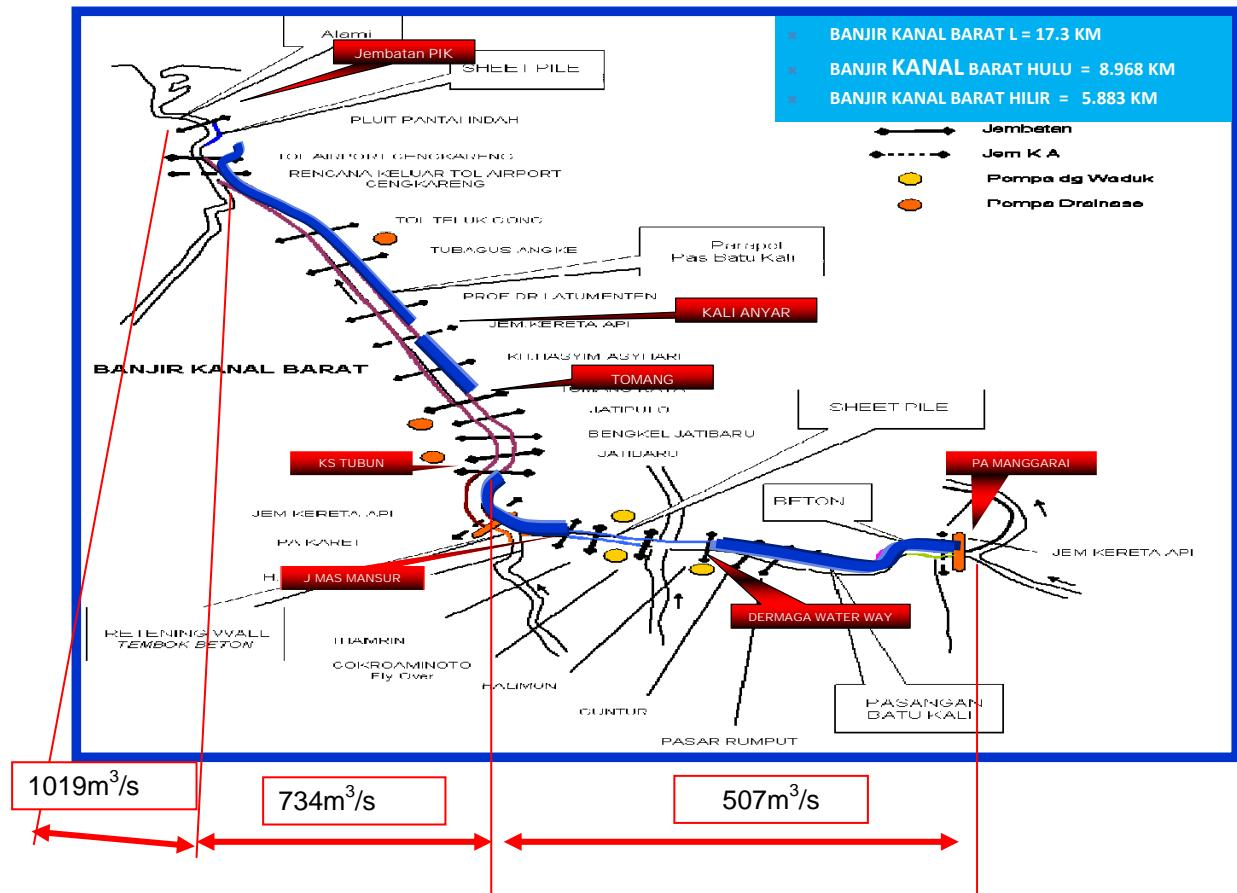
Figure 1.3-1 Improvement and Design Discharge of West Banjir Canal
