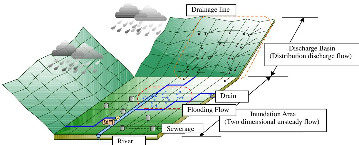
**Figure 3.2-2      Image of Flood Inundation Analysis Model**
