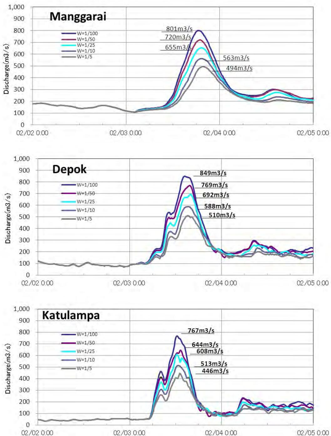
**Figure 3.3-5 Discharge Volume Hydro with Different Design Discharge (Future Land Use, without Inundation, Current River Condition)**
