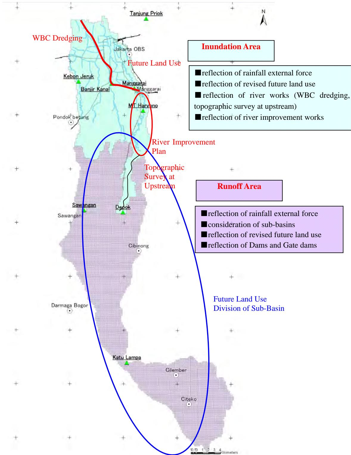
**Figure 3.1-1 Revision of Flood Inundation Analysis Model**
