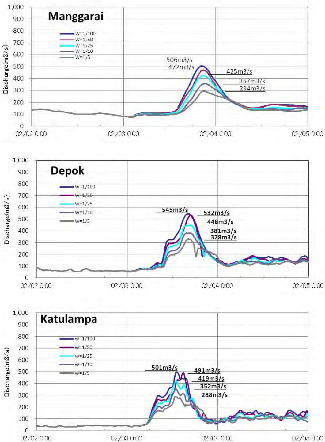
**Figure 3.3-3 Discharge Volume Hydro with Different Design Discharge (Current Land Use, without Inundation, Current River Condition)**
