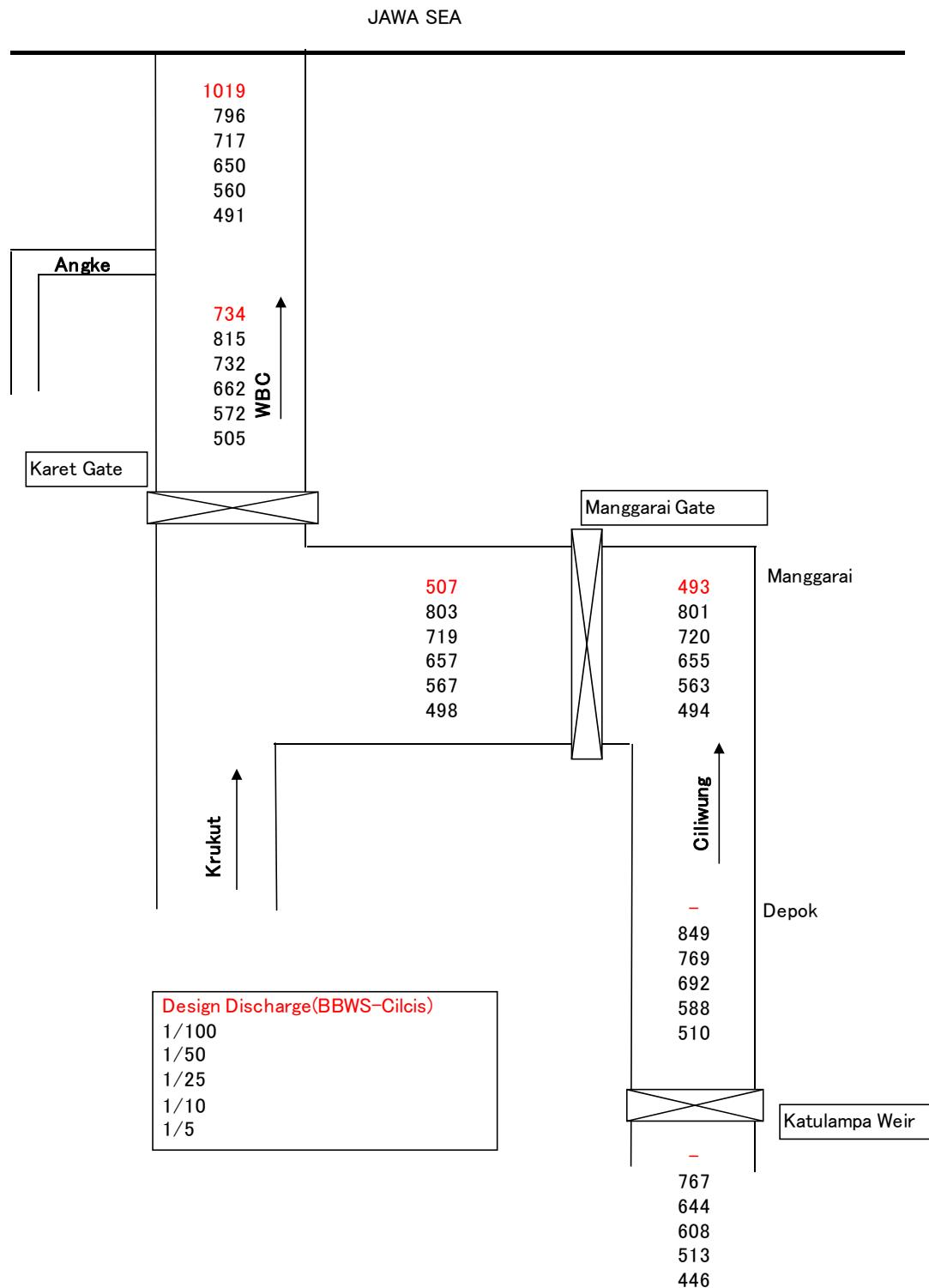
Figure 3.3-4 Discharge Distribution Map with Different Design Discharge
