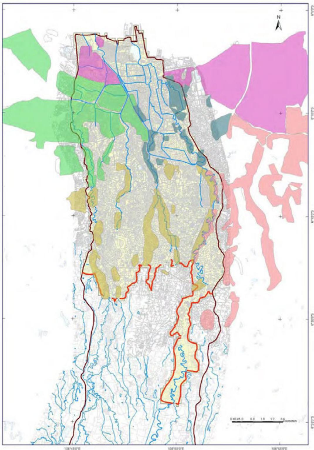
**Figure 3.2-5      Inundation Record Map of 2007 Flood and Inundation Segment**
