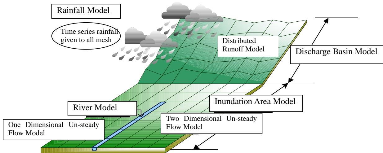
**Figure 3.2-6 Basic Structure of Discharge and Flooding Analysis Model**
