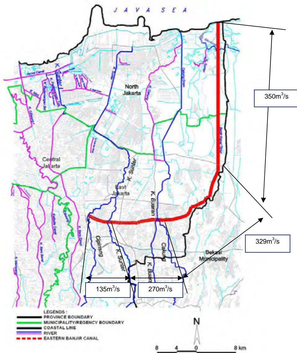
Figure 1.3-3 Improvement Route and Design Discharge Allocation of East Banjir Canal
