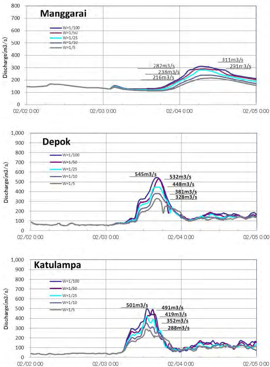
**Figure 3.3-7 Discharge Volume Hydro with Different Design Discharge (Current Land Use, with Inundation, Current River Condition)**
