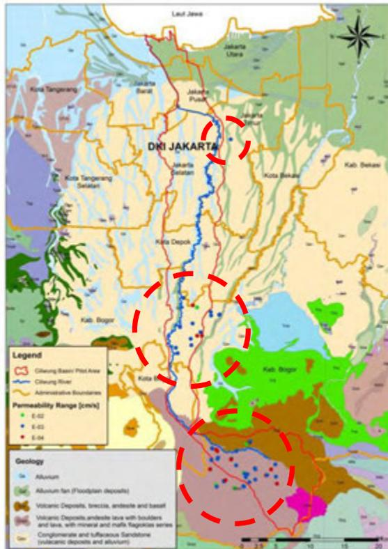
Coefficient of permeability ranges from  $10^{-2}$  to  $10^{-4}$  cm/s. According to the result, most parts of the Ciliung River Basin are suitable for the infiltration facility.
