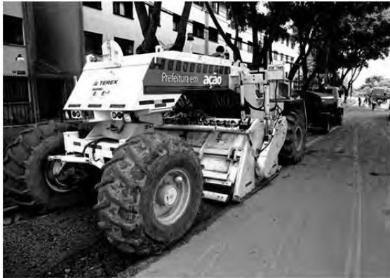
(5) “TEREX RS425C” for milling, recycling and simultaneous application of asphalt pavement
