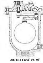
AIR RELEASE VALVE
