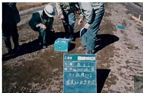
Soil density using nuclear gauge (Radioisotope : RI)
