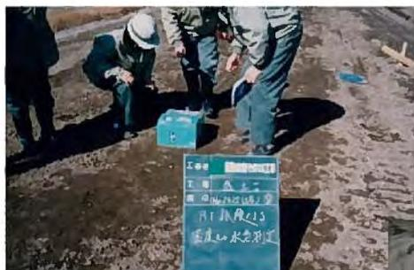
Soil density using nuclear gauge
