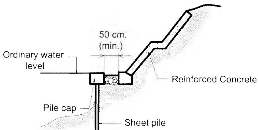
**Allowable Maximum Velocity : Check local scouring depth based on velocity**
