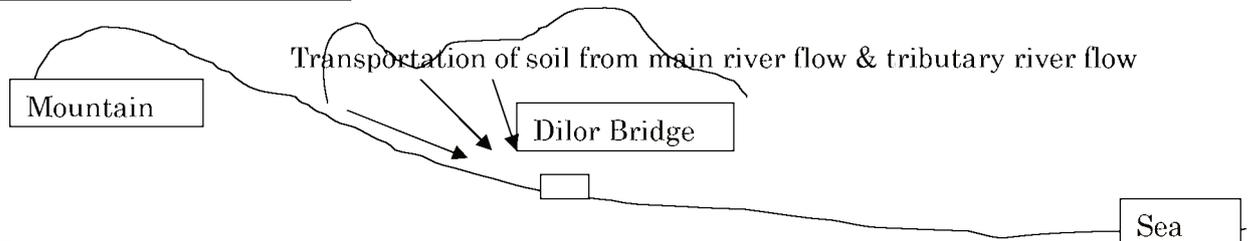
If general sedimentation area, it is necessary to do rising of pier cap. It is difficult to maintain excavation of river bed every year.
