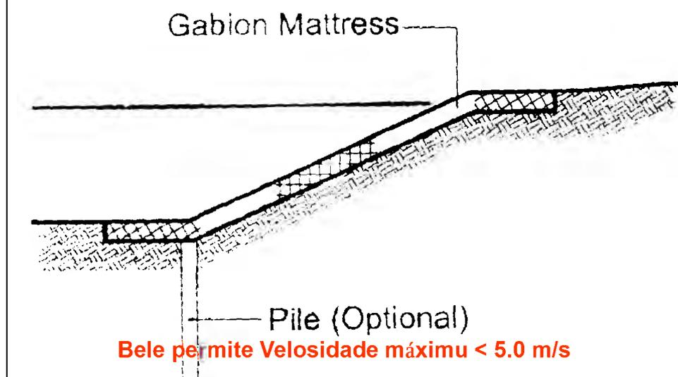
5. Hada-Fatuk Rebokadu/Grouted Riprap, Tipu Expansaun/Spread Type
