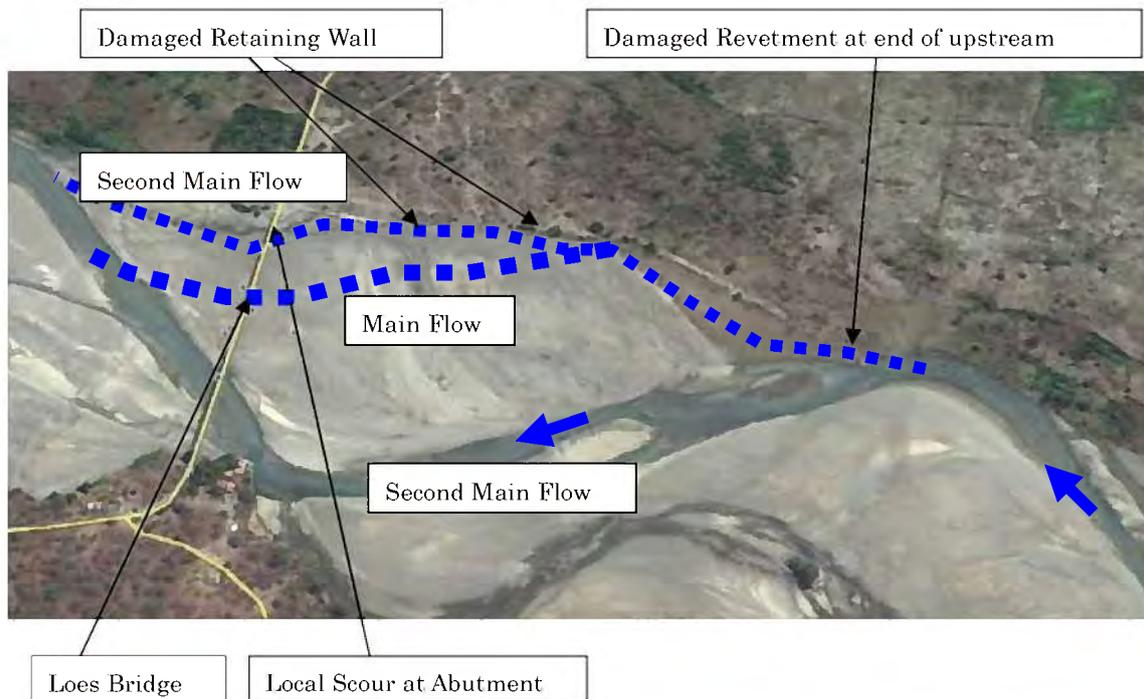
Main flow had shifted at right side from left side on Google map. Second main flow is near abutment and revetment of dike.
