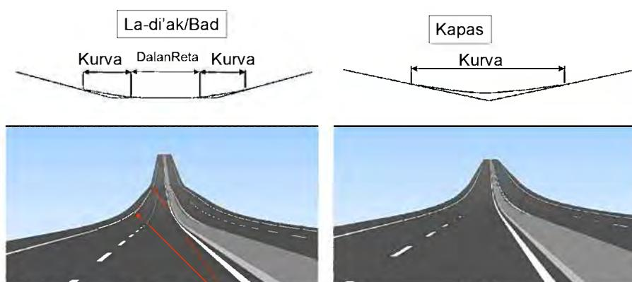
Kurva Kotuk estraga/Broken Back Curve
