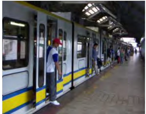
Figure *.12.1 Plug Door of First Generation Train
