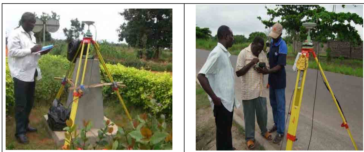
Figure 14 Control Point Survey (Left: Control point origin, Right: Control point)
