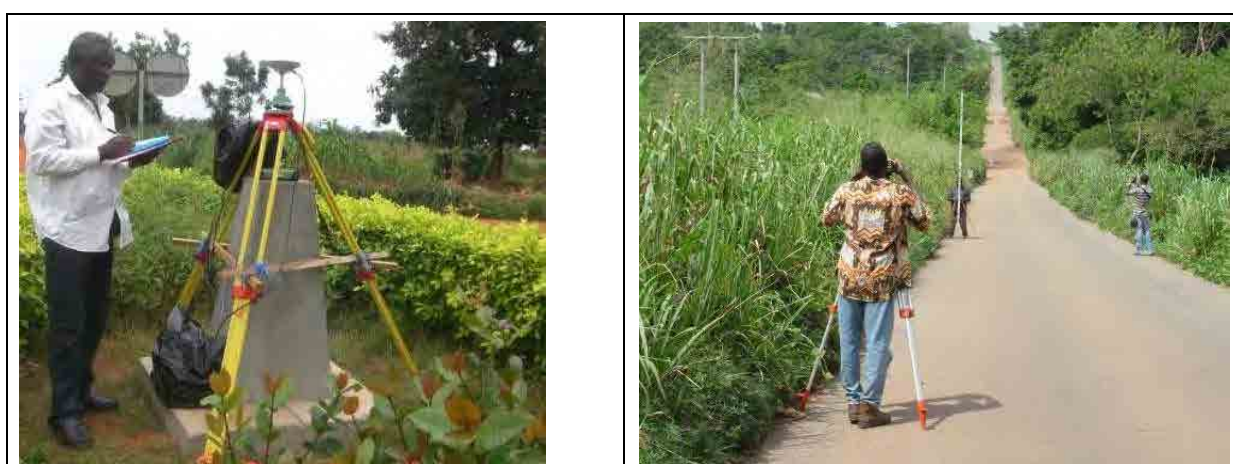
Figure 10 Control Point Survey (Left: Control point origin, Right: Levelling)
