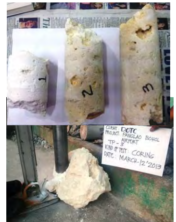
Picture 10.3-1 Core Sample Recovered
