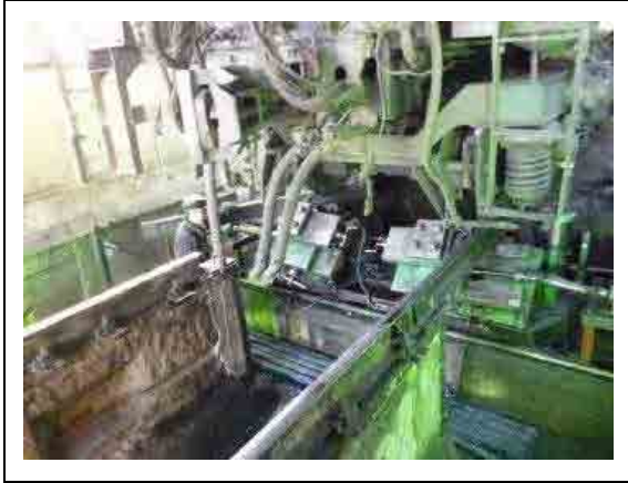
[Fig. 2-32] Wheel Re-profiling Machine
