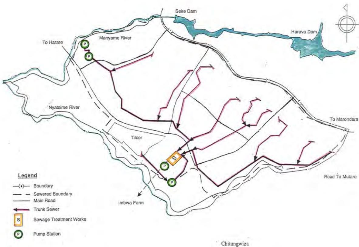
Figure A6.1.4 Sewer Network and Location of STPs in Chitungwiza
