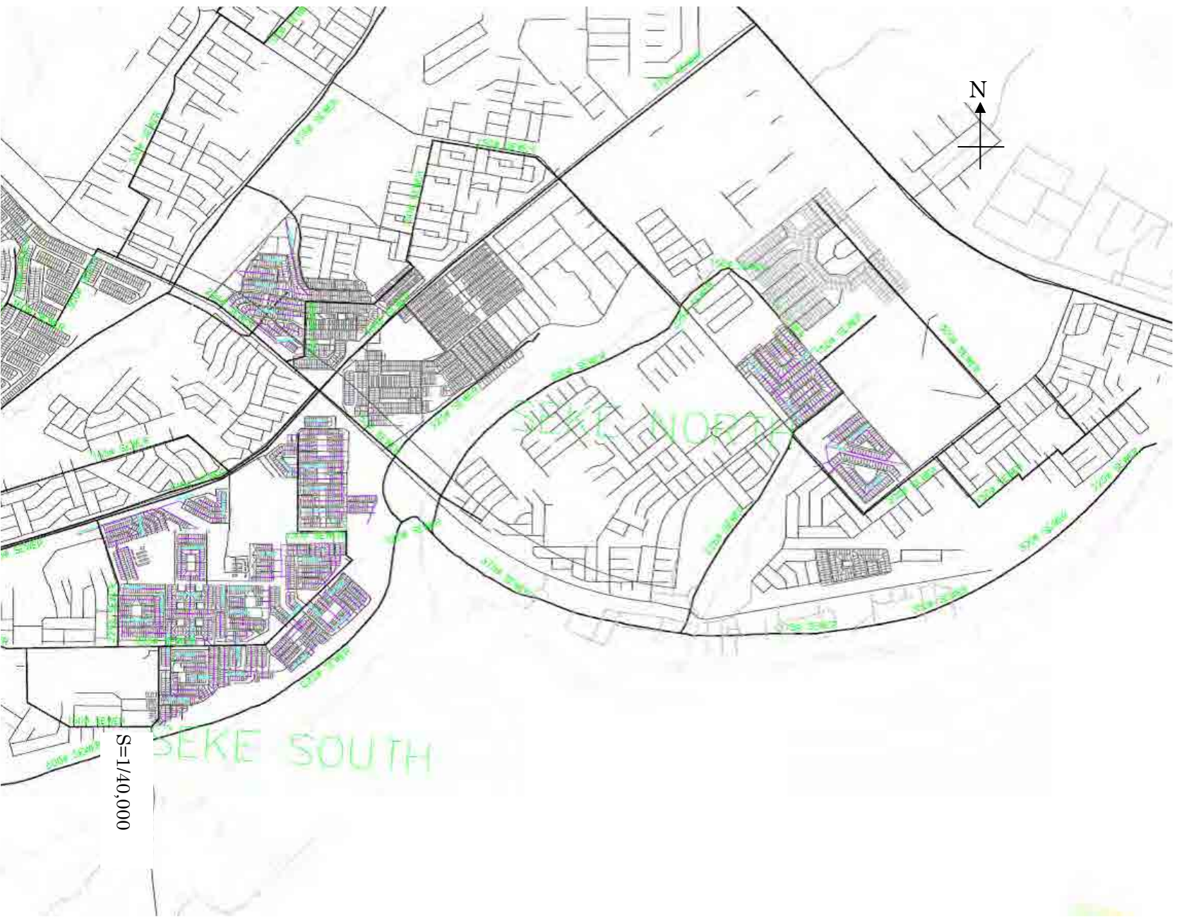
Figure 4.2.5 Sewer Alignment in Seke Area
