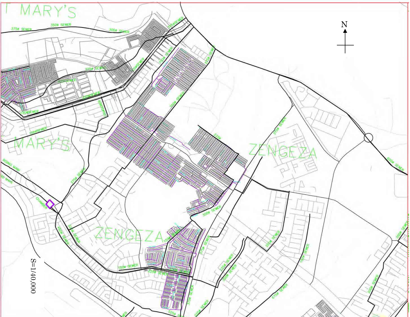
Figure 4.2.4 Sewer Alignment in Zengeza Area
