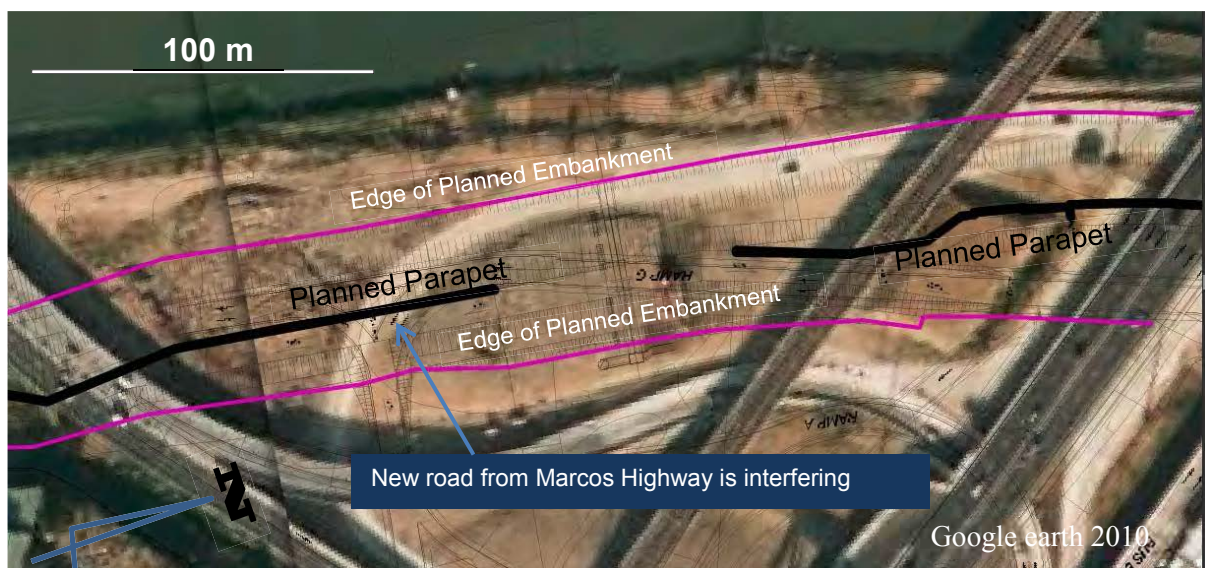
Figure 3.10 Road Interference at Marcos Highway Junction
