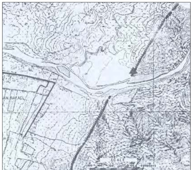
Figure 4.7 Active Fault Lines near Wawa Dam
