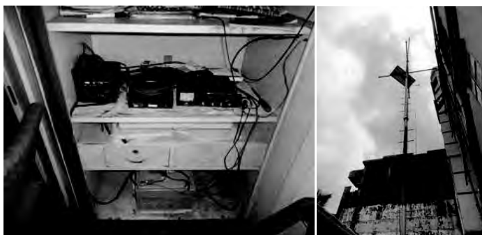
Picture: HF and VHF sets in CPP office and their antenna. CPP team leaders complained that the VHF set is disturbing, they have difficulty understanding messages from it.
