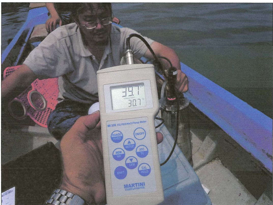
Testing temperature and conductivity on field (19/10/2012)
