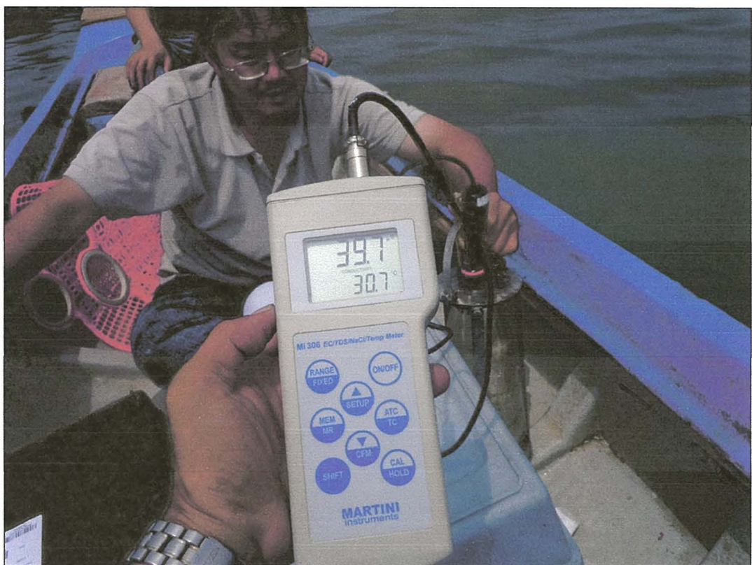
Testing temperature and conductivity on field (19/10/2012)
