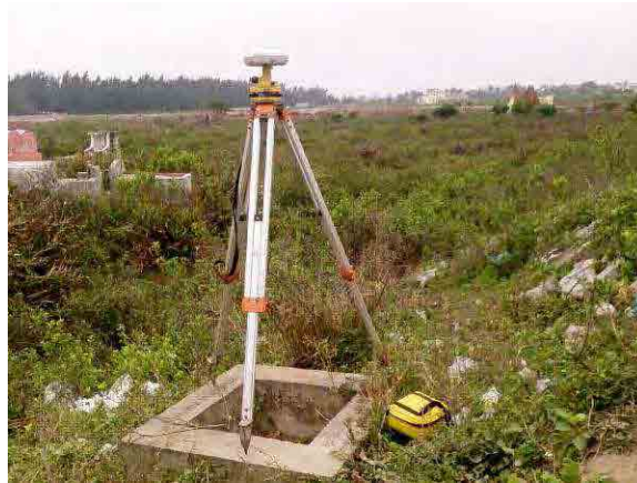
Photo of GPS Measurement National Control Point.
