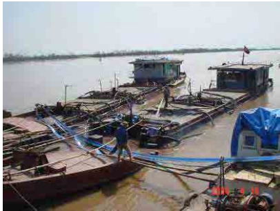
Sand Barge with Pump
