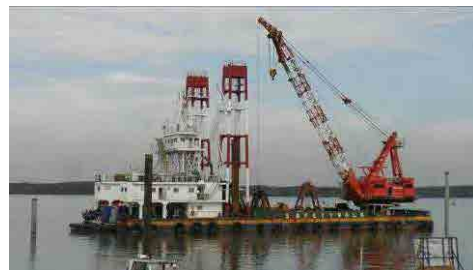
Crane Barge 300t
