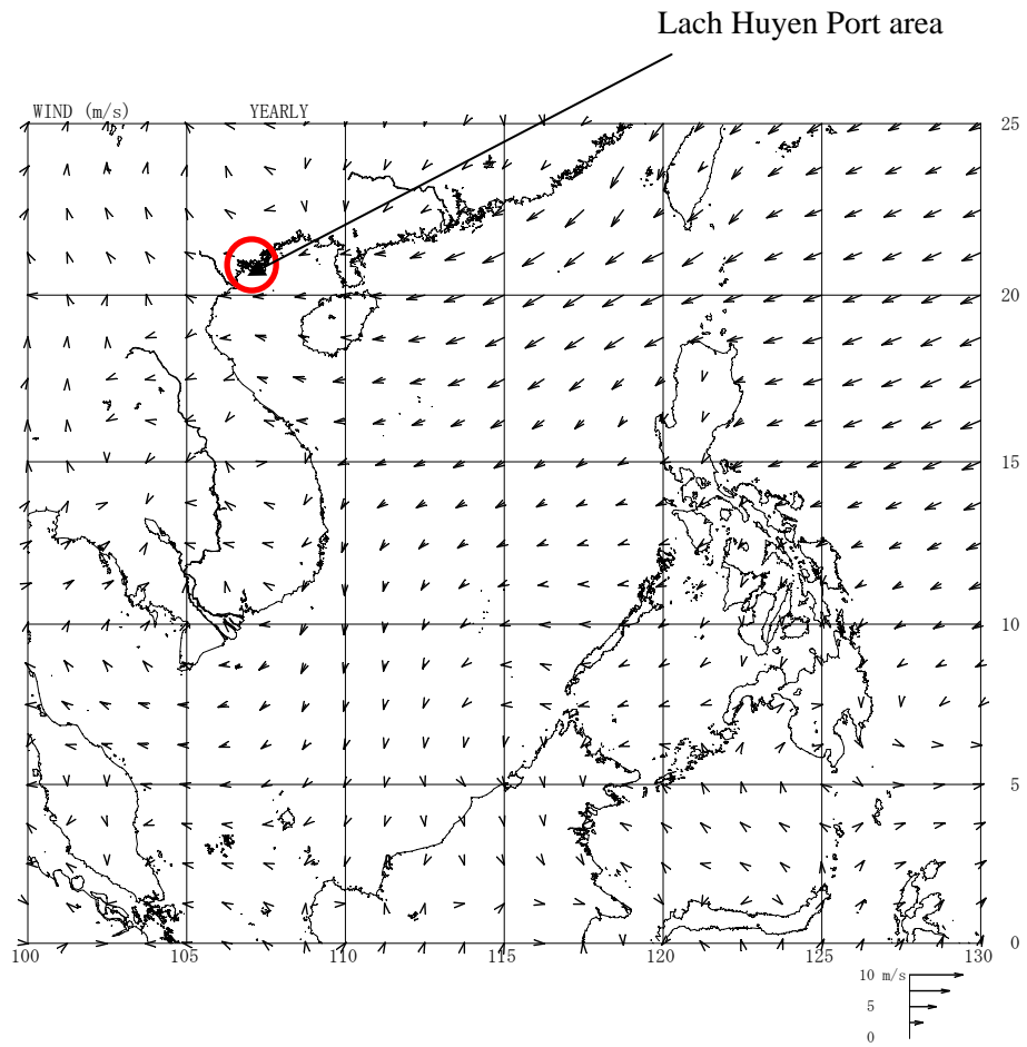
Figure 2.4.1 Horizontal distribution of annually averaged wind vectors based on the global objectivity analysis data published by Japan meteorological agency
