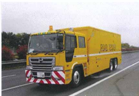
Skid resistance measurement vehicle ; Nippon Expressway Research Institute Co. Ltd.
