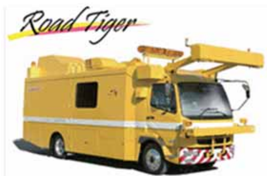
High-speed road surface measurement vehicle 「Road Tiger」 ; Central Nippon Highway Engineering Tokyo Co. Ltd.
