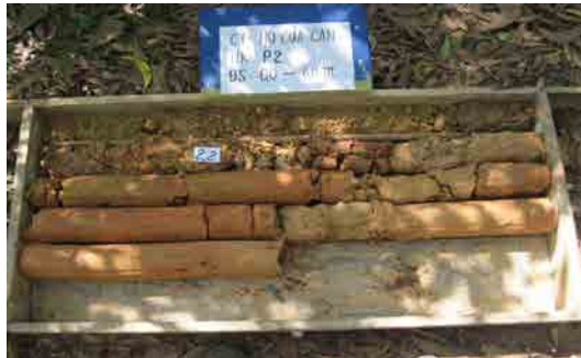
Picture 3-2-2-1 Soils from 0m to 6.0m below ground
