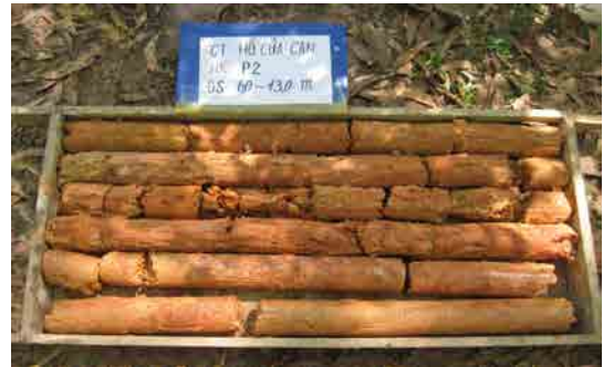
Picture 3-2-2-2 Soils from 6.0m to 13.0m below ground
