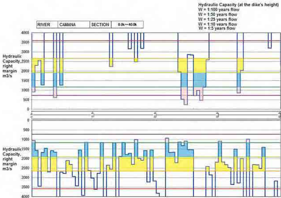
Figure 3.1.10-3(2) Current discharge capacity of Camana River
