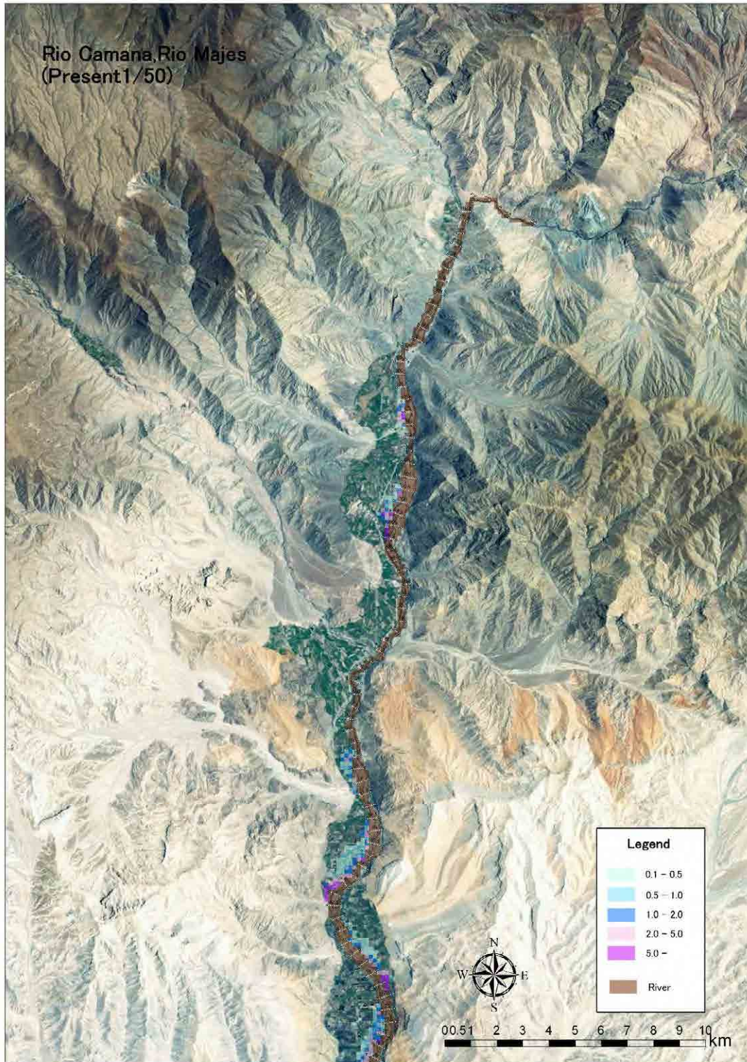
Figure 3.1.10-4(1) Inundation area of Majes-Camana river
