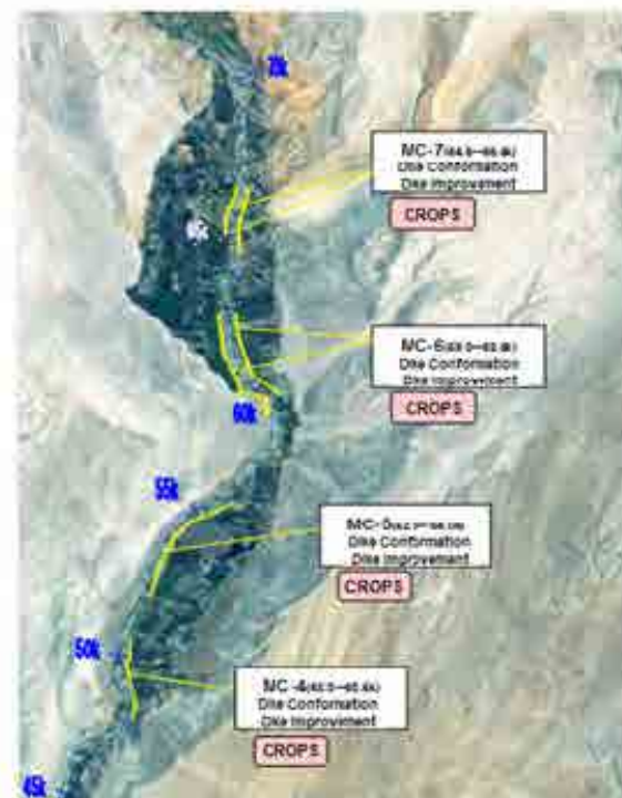
Figure 4.3.1-4 Prioritized flood control works in Majes river
