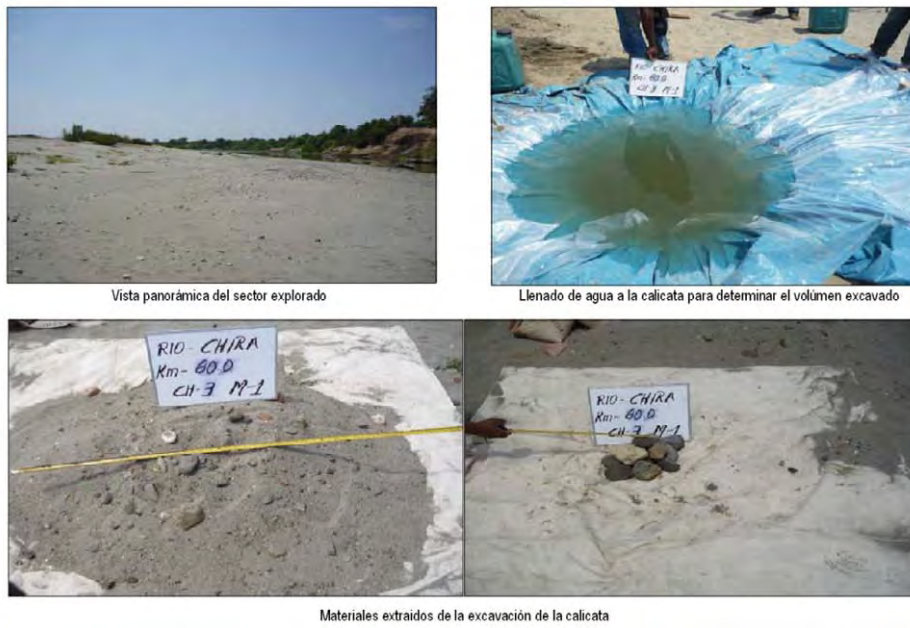
Figure 1.11 Riverbed Material Sampling Survey (Chira River No. 3)
