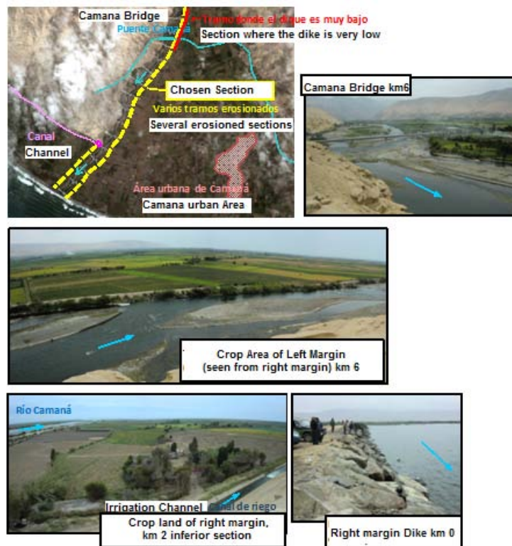
Figure 3.1.6-3 Local conditions related with Challenge 1 (Camana River)
