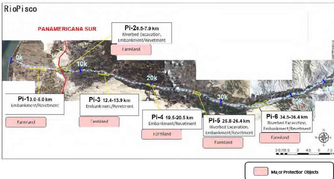
Figure 4.3.1-10 Prioritized flood control works in Pisco river
