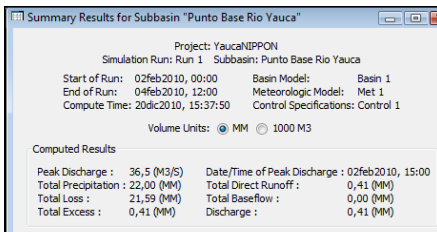
Figure N° 4.13. Results Model Simulation of Rainfall – Runoff Yauca River, Return Period of 5 years
