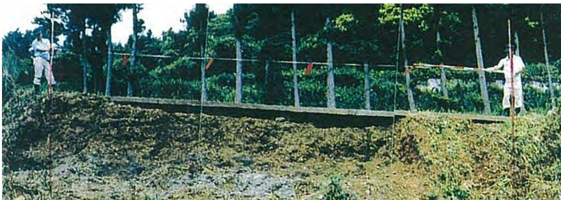
Photo 2.2.1 example of measuring the length of damage using poles and a tape measure (together with red cloths)
