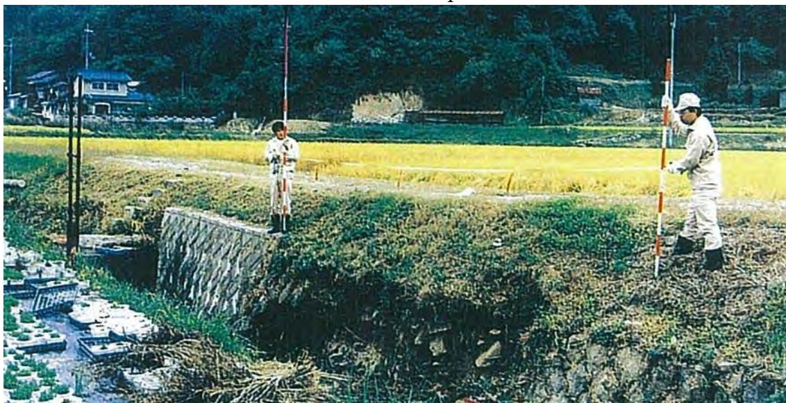
Photo2.2.5 Example of measuring the length of damage using poles and tape measure (together with red cloths)
