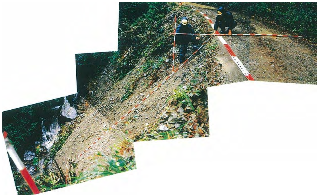
Photo2.2.13 Measurement when a slope is stable
