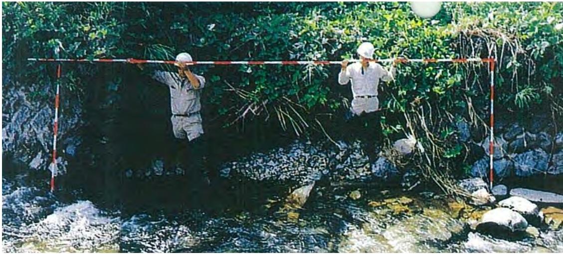
Photo 2.2.3 Example of measuring the length of damage using poles
