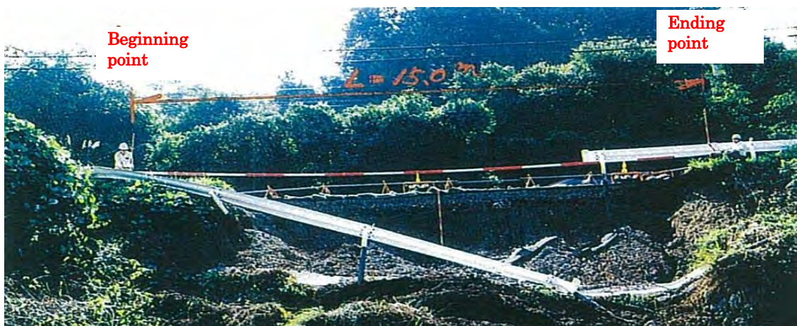
Photo 2.2.2 Example of measuring the length of damage using poles and ribbon rod (1m pitch)
