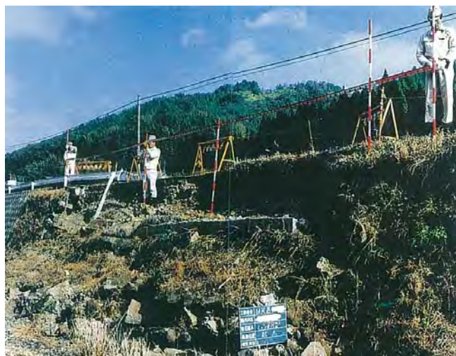
Photo 2.2.4 Example of measuring the length of damage using poles and ribbon rod (1m pitch)
