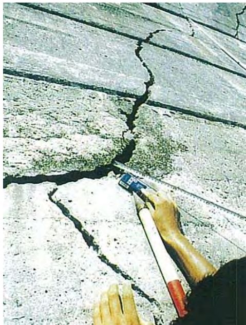
Photo2.2.16 Measuring cracks on a concrete retaining wall
