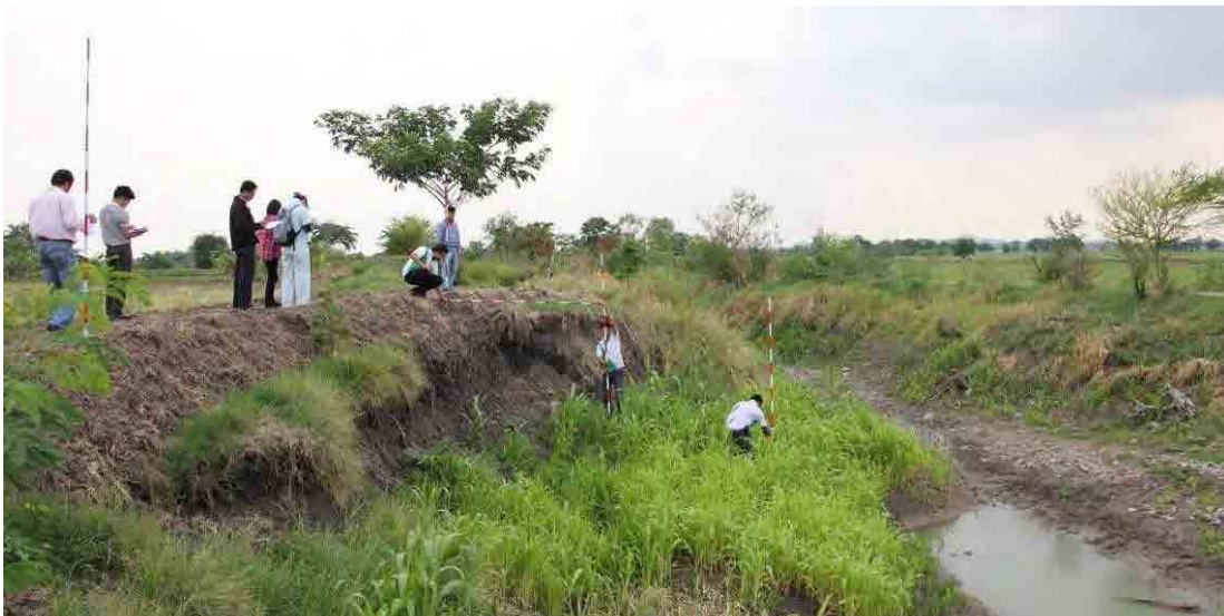
Photo 8.1-4 The measurement of the flood damage change point section with the pole
