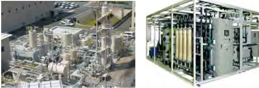
Photo 225- 1 Feed-water treatment system
